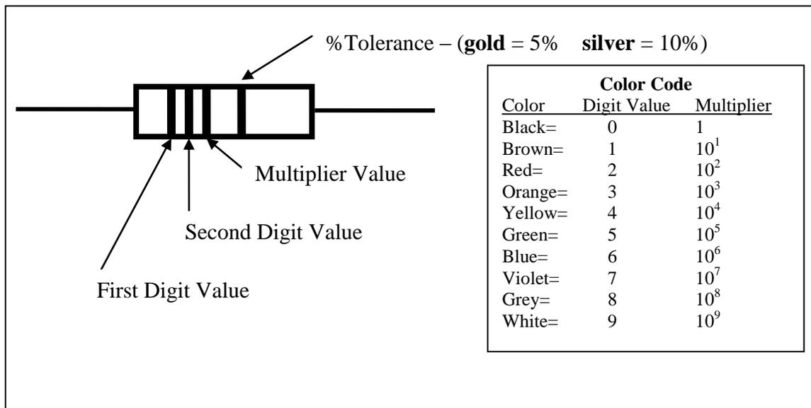
**Figure 1:** The farthest left non-metallic band is the first digit value, the second band is the second digit value, and the third band is the multiplier value. The fourth band indicates the accuracy of the resistor – which will be discussed later in the lesson.
