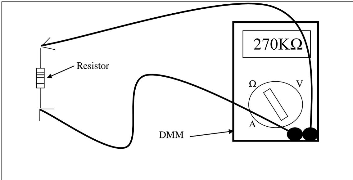
**Figure 2:** Connect your black test lead into the “COM” or common terminal and your red test lead into the “V, Ω” terminal. Set the circular dial selector to the resistance or  $\Omega$  setting on your DMM. Lay the resistor flat on the desktop and make good contact with the resistor. Do not poke yourself or your partner in this process.
