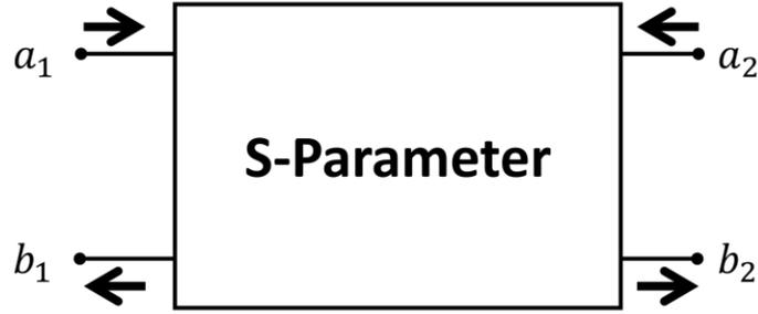
Figure 5.6 – S-parameter for two port RF MEMS network.
