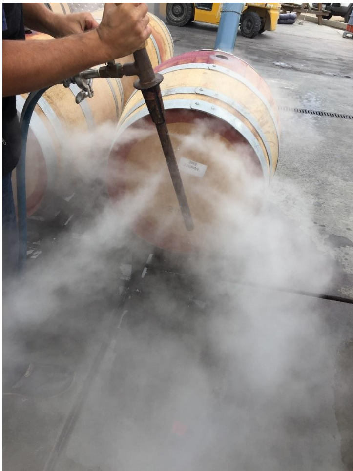
Figure 10. Steam cleaning barrels. To save water, wineries use steam and pressure to keep their wineries immaculately clean. Cleanliness prevents unwanted organisms from damaging the wine. Photo by author.
