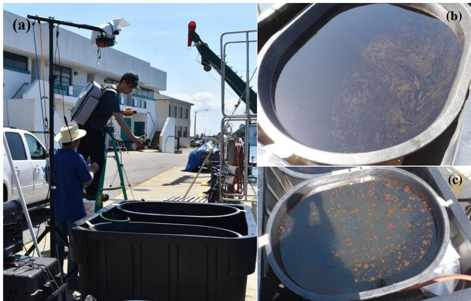
Figure 5. 1: a) Oil experiment in a water tank by the USF College of Marine Science campus seawall in St. Petersburg, Florida. Shaojie Sun and Chuanmin Hu were measuring the oil spectral reflectance using the SR-1900 spectrometer (photo credit: George Graettinger). Two identical tanks were set side by side, each other with same volume of b) crude oil and c) oil emulsions.
