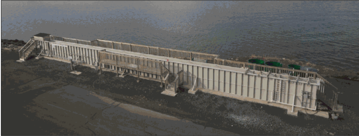
Figure 2.1. The wave tank facility at Bedford Institute of Oceanography. Dimensions: 32 m long, 0.6 m wide, and 2 m high (1.5 m water depth; 28,800 L volume). Breaking and non-breaking waves generated by a computer-controlled flat-type wave maker situated to provide mixing energies and achieve dispersant effectiveness observed in the field. Reprinted from “Submersible Optical Sensors Exposed to Chemically Dispersed Crude Oil: Wave Tank Simulations for Improved Oil Spill Monitoring,” by R.N. Conmy, et al., 2014, Environmental Science & Technology , 48, p. 1803. Copyright 2014 by American Chemical Society. Reprinted with permission.
