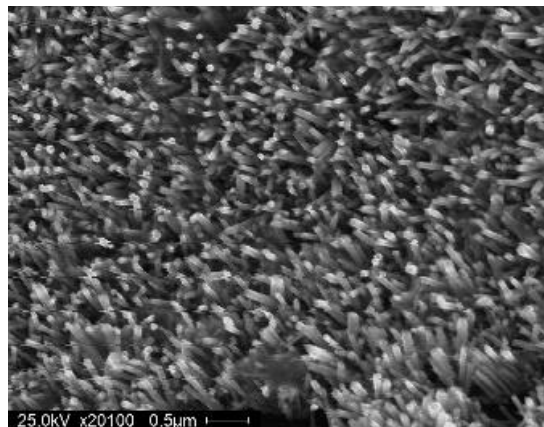
Figure 37. SEM image of the hydrothermally grown ZnO nanowires on an ITO substrate.
