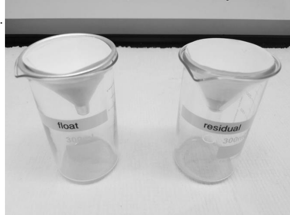
Figure C.1: Two labeled beakers set up for the trichloroethylene procedure
