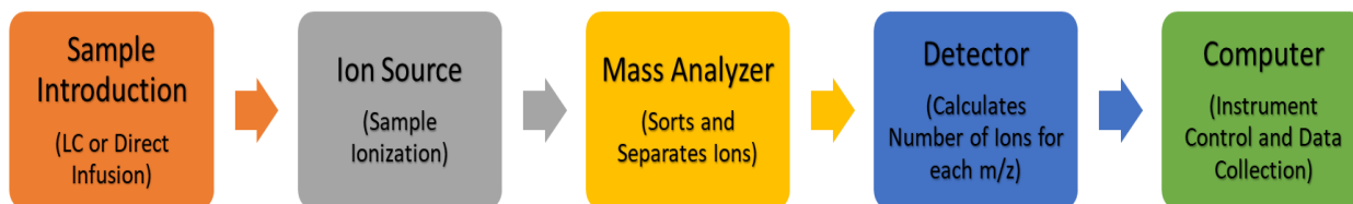
Figure 1.6: General Overview of LC-MS Analysis. Sample is resuspended in HPLC-H 2 O and loaded onto the LC where it will bind the separation column. As organic solvent is increased, the peptides eluting off the column will be ionized into the gas phase. The mass analyzer will next separate the precursor ions on mass to charge. In tandem MS, the precursor ions can then be further fragmented by CID into daughter ions. The detectors calculates the number of ions for each peptides and the computer records the data as relative abundance and/or intensities.
