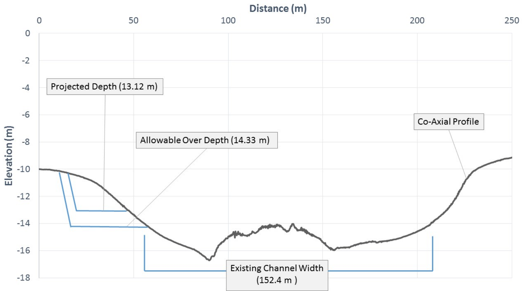
Figure 2. Plans for 30 m channel-widening beneath the Skyway Bridge, depicted on a representative co-axial profile of the shipping channel. Elevation is relative to MLLW.
