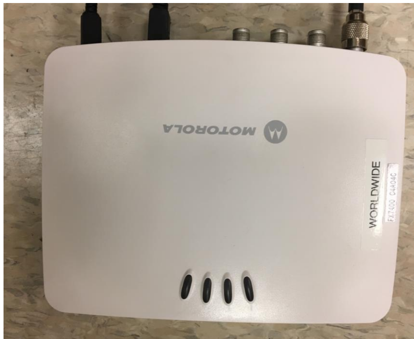
Figure 5.2 A photo of fixed RFID reader.
