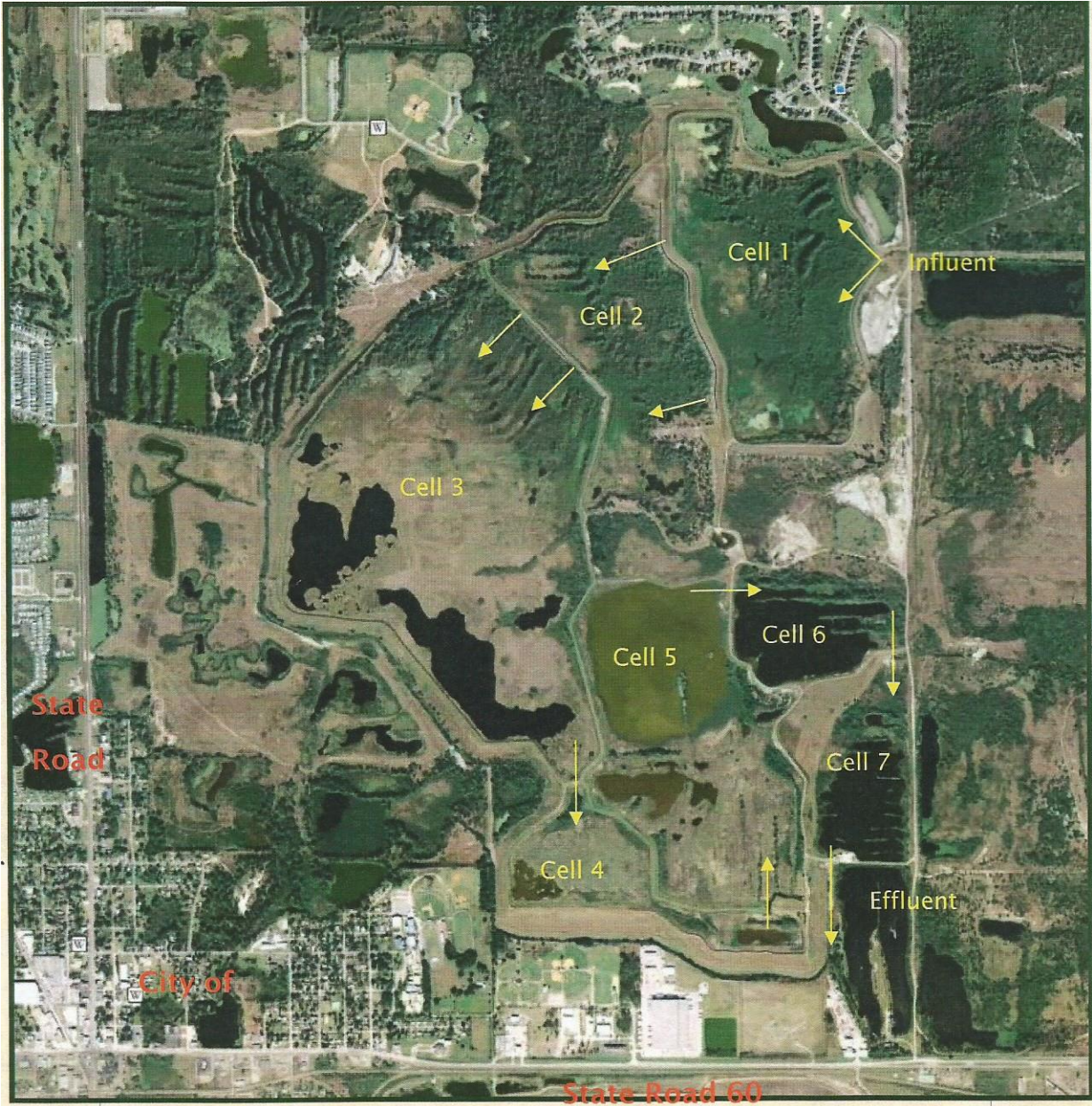
Figure 5: The City of Lakeland’s Wetland Treatment System Flow Patterns (City of Lakeland, 2015)
