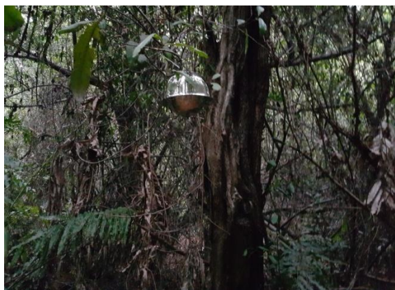
Figure 3.4: Polyurethane foam passive air sampler mounted in the forest
