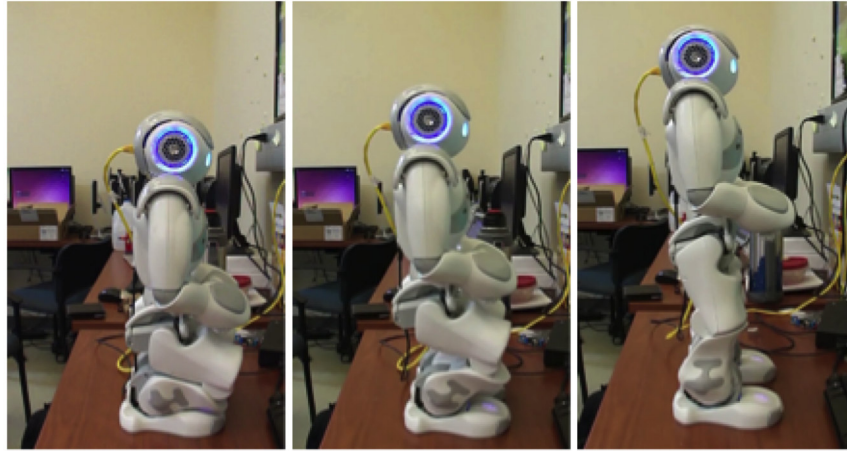
Figure 2.7: NAO robot performing stand up movement using reduced stiffness levels.
