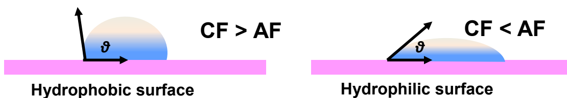
Figure 3.3 Illustration of the interplay of Cohesive Forces (CF) and Adhesive Forces (AF) of a water droplet on a hydrophobic vs hydrophilic surface.
