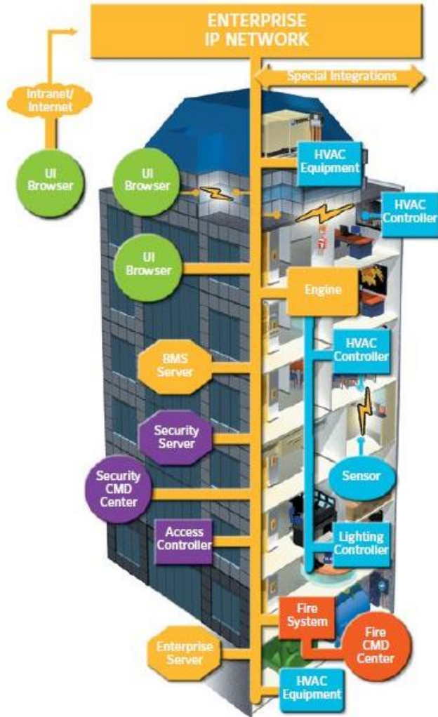
Figure 1-2: BAS Network Infrastructure. Source: http://www.johnsoncontrols.com/
