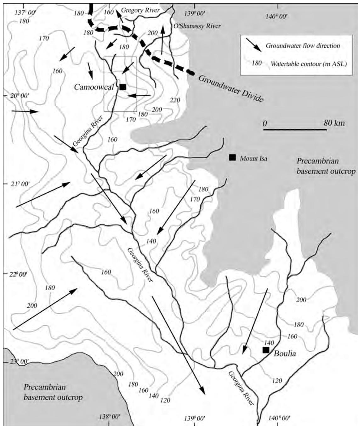
Figure 1. Southeastern Georgina Basin, showing surface drainage, watertable contours and inferred groundwater flow directions, including the groundwater divide inferred to exist between the headwaters of the Georgina River and Gregory–O'Shanassy Rivers. The Camooweal karst area (see Figure 2) is the area inside the box. Adapted from Randal (1978).
