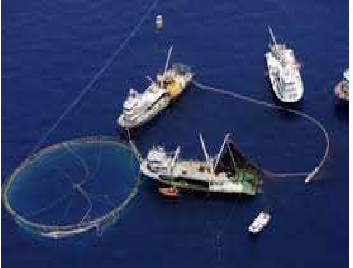
Figure A14. Aerial view of purse seine net fishing. Purse seining is normally used to encircle entire schools of pelagic species such as tuna.
