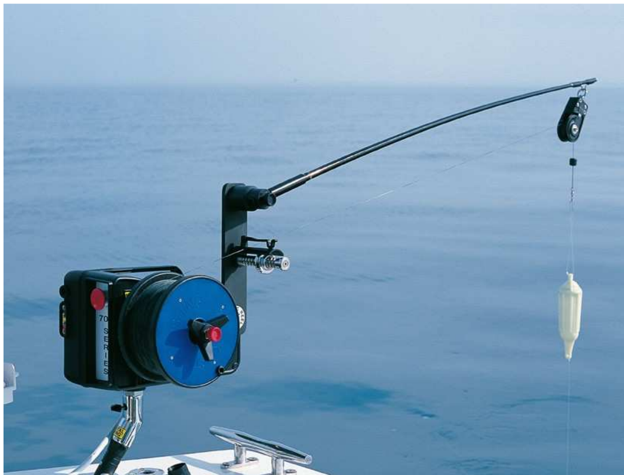
Figure A2. Bandit fishing reel. Electric or hydraulic reel used in commercial fishing to target bottom dwelling fish, such as grouper and snapper. Illustration above shows an electric bandit reel rigged with a light stick to attract fish to the baits. Below the white light stick is a 12-foot wire leader with 4 to 10 baited hooks with a lead weight attached to the end of the leader to allow the baited hooks to remain on the bottom.
