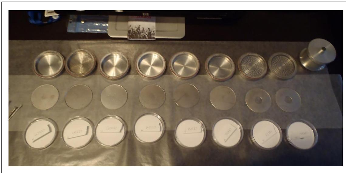
Figure 7. Andersen Cascade Impactor disassembled – SSS1. Stages of the cascade impactor are shown laid out across the top; stainless steel plates are shown in the middle; 81 mm glass fiber substrates are shown in Petri dishes on the bottom. The pre-separator is shown in the upper right hand corner of the photograph.
