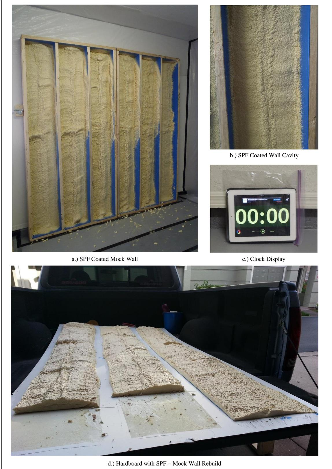
Figure 13. SPF application. a.) Mock wall sections insulated w/SPF. b.) Close-up of SPF filled cavity. c.) Time display used for surveys. d. SPF adhered to hardboard during mock wall rebuild.
