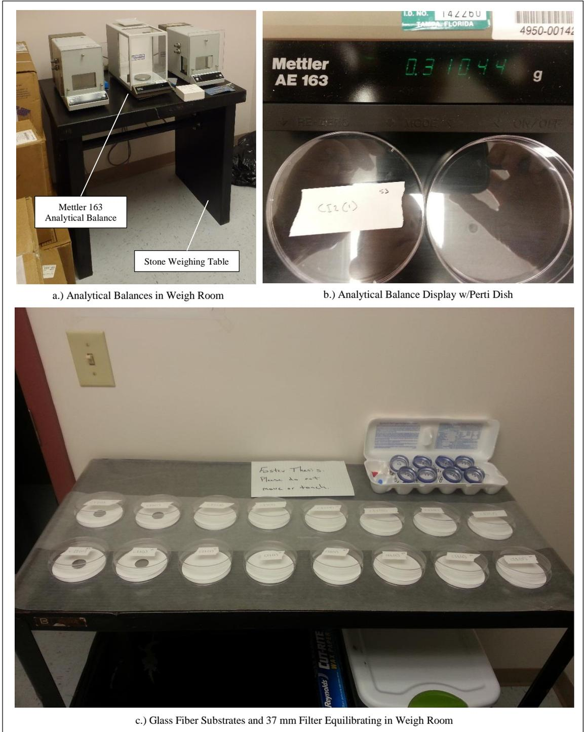
Figure 5. Analytical balances and filters/substrates in weigh room. a.) Analytical balance used for Surveys 1-3 shown in the middle – Mettler Model 163. b.) Display of balance shown under load. c.) 81mm glass fiber substrates for cascade impactors and 37 mm filters for total dust.
