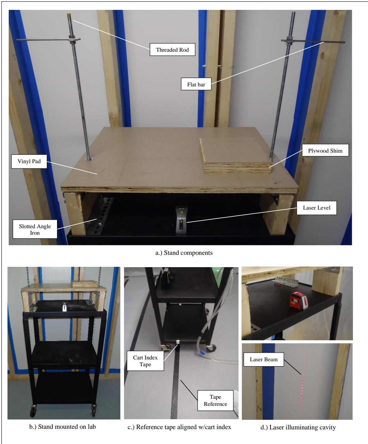
Figure 4. Laboratory cart modified w/stand. a.) Stand with components described. b.) Stand shown mounted on top of lab cart. c.) Lab cart shown aligned with tape reference on the floor. d.) Laser level powered on casting vertical beam on the center of the wall cavity
