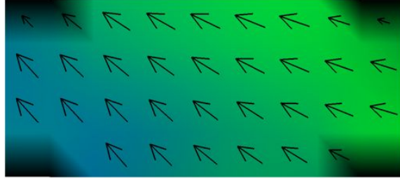
Figure 4.19. Intermediate magnetization state of clocked cell with tilted polarizer
