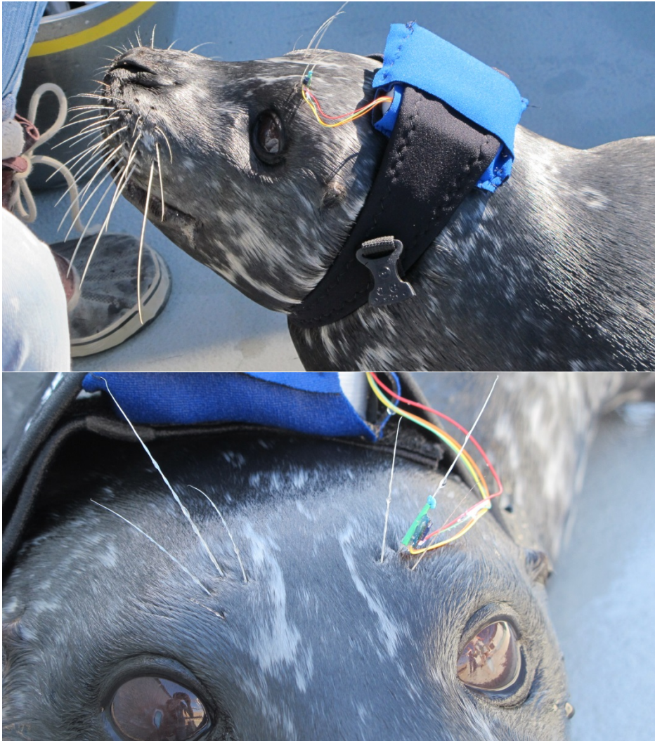
Figure 3.5 Photographs of the trained harbor seal wearing the wLogger tag. The accelerometer is attached to a supraorbital whisker. The main recording unit is fitted to the animal's head by placement inside a pocket of the neoprene headband.
