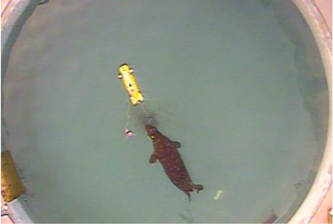
Figure 3.6 Photograph of the seal tracking a radio-controlled submarine while wearing the wLogger tag. This photograph was obtained from the overhead video camera system used to synchronize tag recordings to behavioral events.
