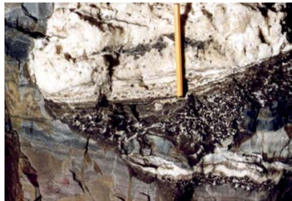
Fig. 12. Base of filled passage, revealed after calcite mining. Note wad fragments (black) detached from the wall representing phreatic residual, in calcite matrix subsequently deposited in the vadose zone, overlain by flowstone. Note discontinuity with dolostone. Pen as scale. In passages to the SW of Elephant Chamber.
