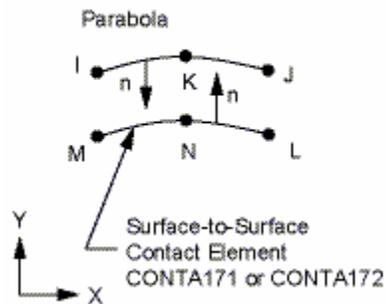
Figure 10: Structure of the TARGE169 element (ANSYS)
