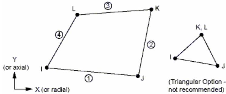
Figure 7: Structure of the PLANE182 element (ANSYS)
