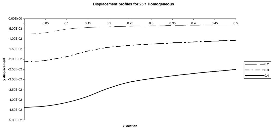
Figure 15: Sample displacement profiles for  $a/T_f$  values of 0.2, 0.3, and 0.4
