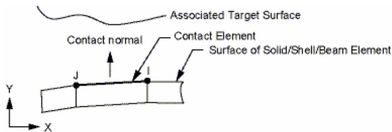
Figure 9: Structure of the CONTA171 element (ANSYS)
