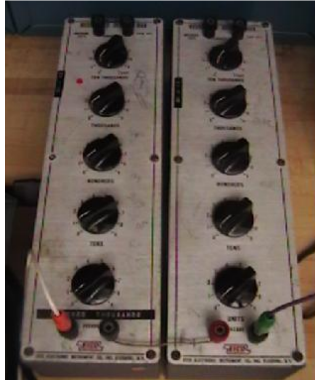
Figure 17: Two Resistance Decade Boxes Wired in Series.
