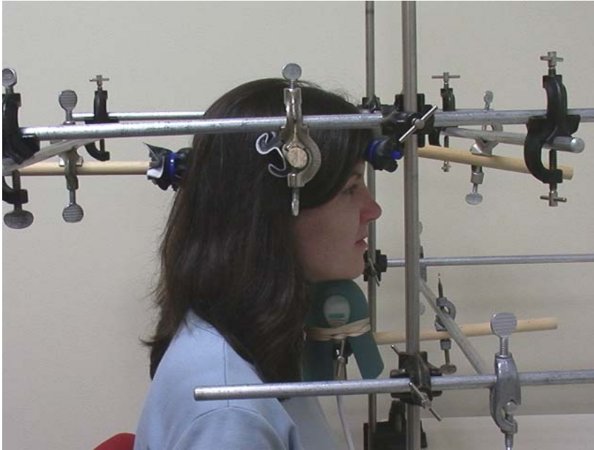
Figure 2 Cushion-scanning technique within head stabilizing frame
