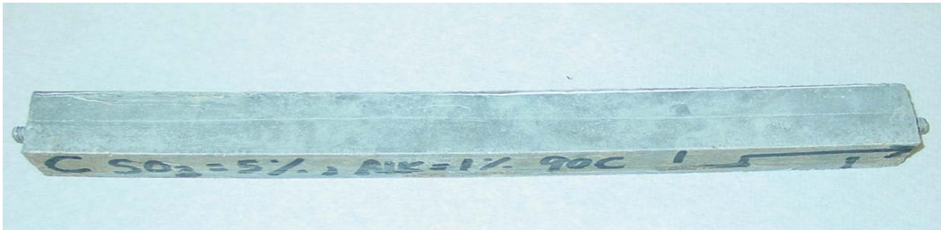
Figure 2: Mortar bar showing bending
