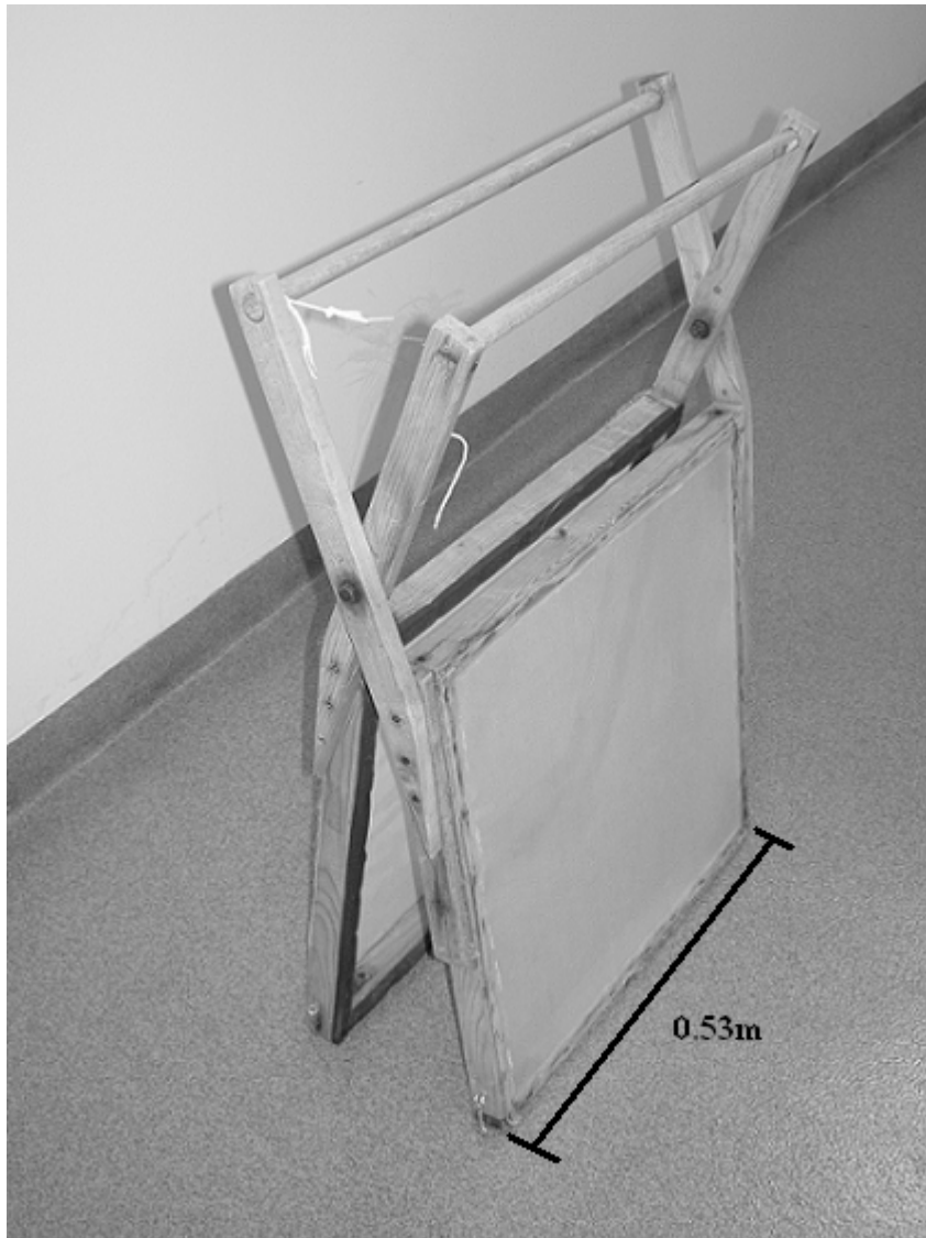
Figure 2. View of the X-sampler used to collect epifauna samples, in the open position.
