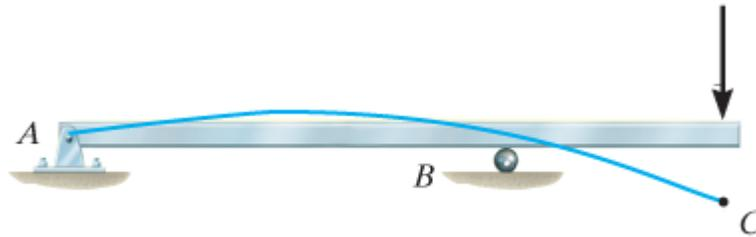
determine the displacement of the overhanging end of the beam if the beam is loaded at its overhanging end.
