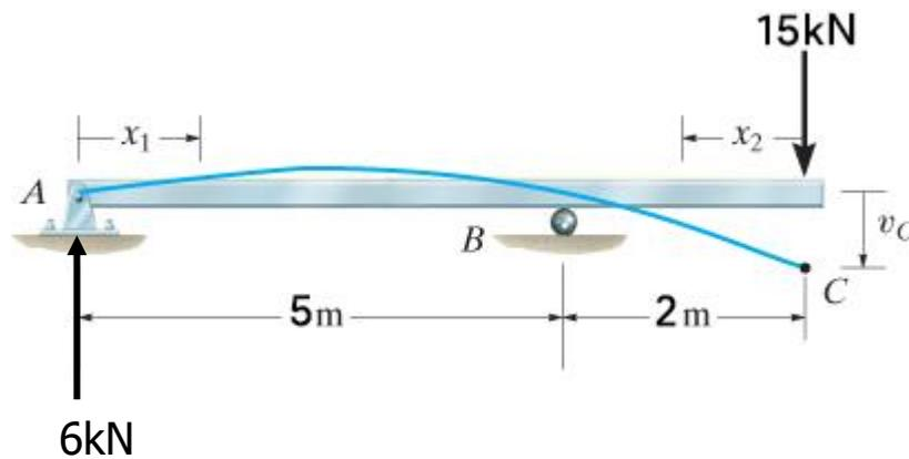
Figure 2: Overhanging beam with correct given information
