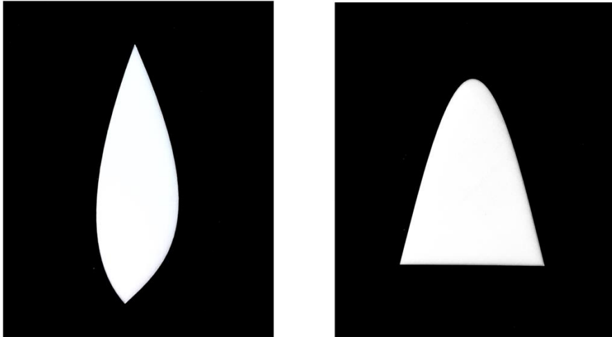
Figure 10: The 3-D printed models of geometric regions bounded by f(x) = \sqrt{x} with g(x) = x^3(1) and f(x) = 2\sin 2x (2)
