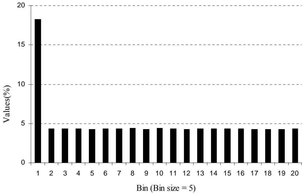
Figure 4.7 – Histogram of Packet Delays – Poisson Traffic
