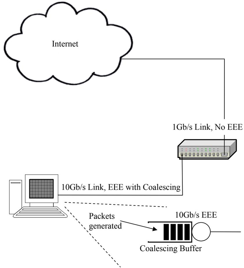
Figure 3.7 – High-Level Illustration of EEE with Packet Coalescing
