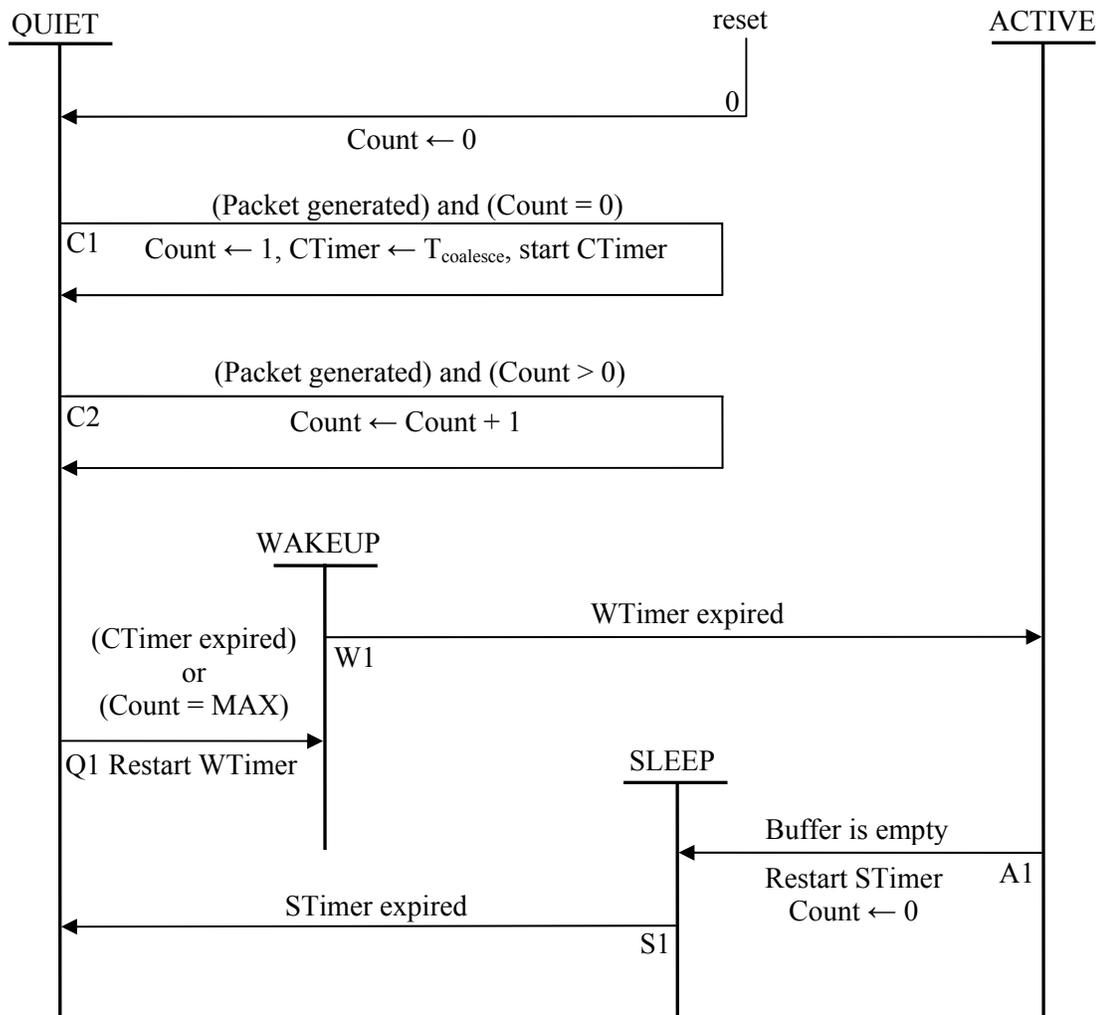
Figure 3.5 – FSM for EEE with Packet Coalescing
