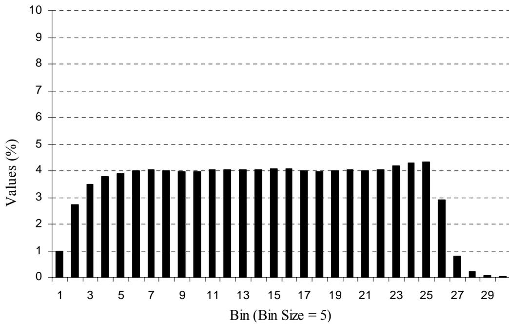
Figure 3.13 – Histogram of Packet Delays (90% Load, Large Coalescer)
