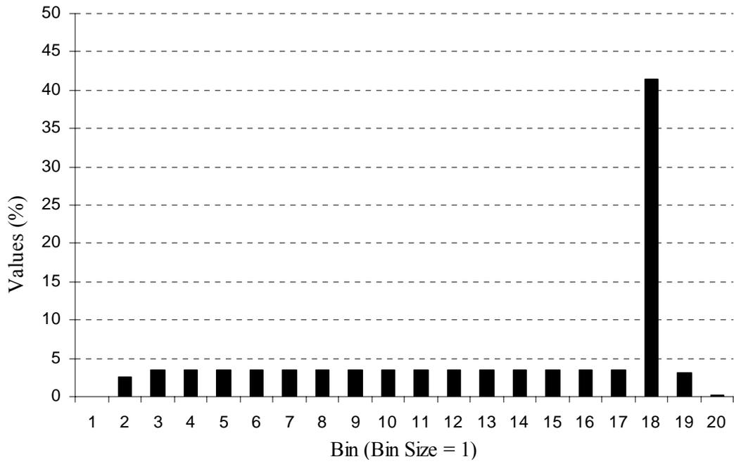
Figure 3.10 – Histogram of Packet Delays (10% Load, Small Coalescer)
