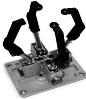
**Figure 1:** A four fingered robotic hand.
