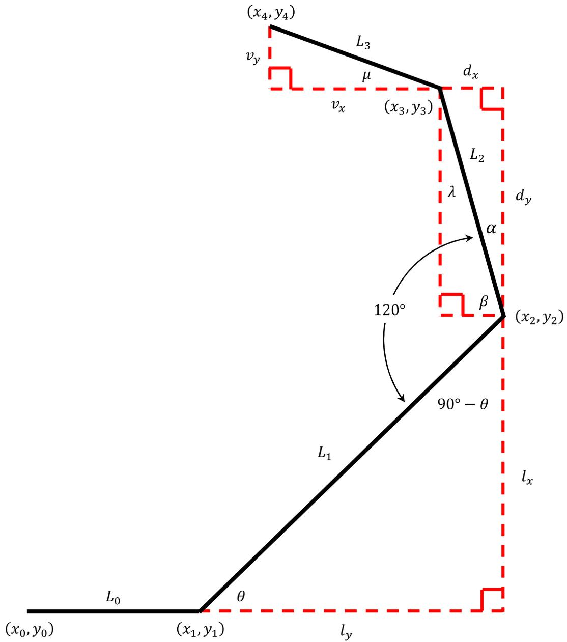
**Figure 2:** This figure illustrates the basic setup for the robotic finger. The finger is divided into four segments:  $L_0$ ,  $L_1$ ,  $L_2$ , and  $L_3$  of lengths 4", 10", 7", and 4", respectively.
