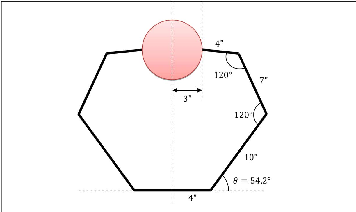
**Figure 3:** In the initial setup, the robotic hand holds a ball of radius 3" in space. The angle  $\theta$  which achieves this position is 54.2°. The distance from the center of the ball to the base of the hand is calculated to be 18.5".
