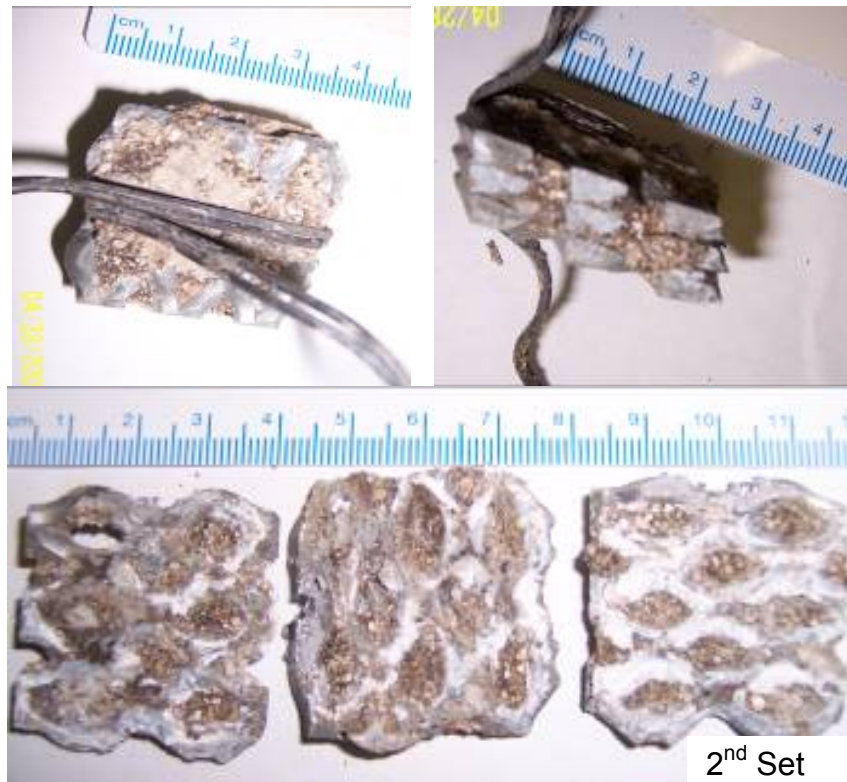
Figure 3 - Type W anode specimens. Zinc alloy anode appearance after embedded mortar was stripped. Top 1st set. Bottom 2nd set. (Mortar only partially stripped).
