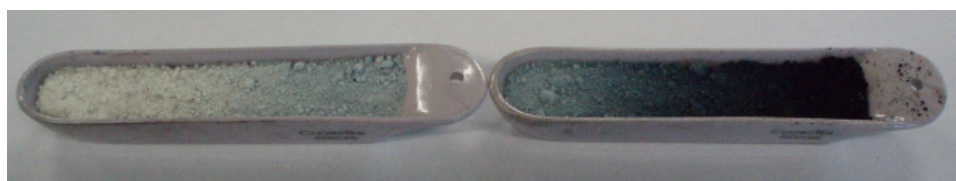
Figure 63 Thermochemically Ammonia Treated Degussa P-25 TiO 2 at 675°C at 87.3 mL/min. for 3 Hours
