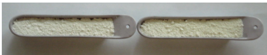
Figure 60 Thermochemically Ammonia Treated Degussa P-25 TiO 2 at 675°C for 3 Hours at 12.7 mL/min.
