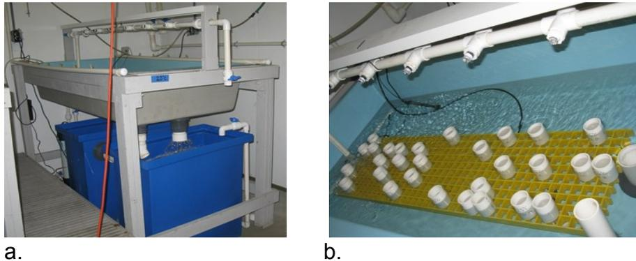
Fig 2. (a) Water table structures, with recirculating water, and (b) raceways in water table with microcosms and heater.
