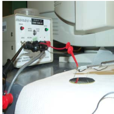
Figure 5.18 Poling Set-Up Using DC Probes
