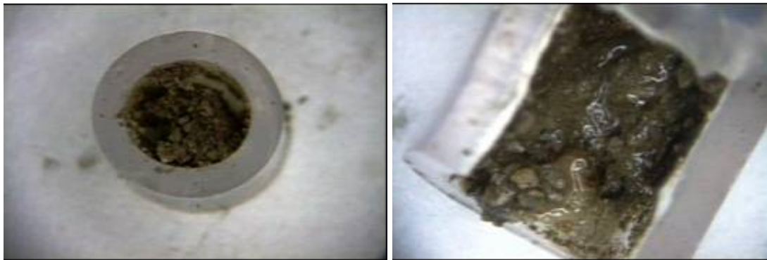
Figure 9. Photograph of Deposits in Leachate Collection Tubing from a.) MSW Monofill Lysimeter, and b.) Co-disposal Lysimeters. Tubing has an ID of 8 mm and OD of 10 mm.
