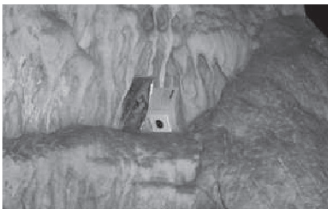
Fig. 5 - An etched track detector in place (Grotte di Toirano, Italy).
