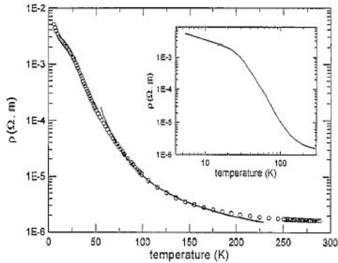
**Figure 2.1.1** Resistivity dependence on temperature of FeSi bulk material. [Mihalik et al., J. Magt. Magt. Mater, 1996].
