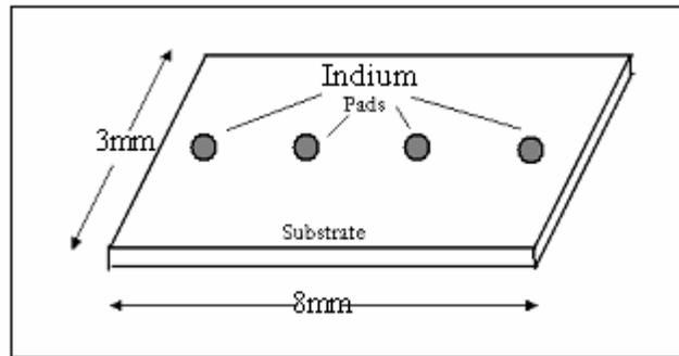
**Figure 4.1.2:** Schematic Diagram of the sample used for Resistance Vs. Temperature (RT) and current vs. voltage (IV) measurements
