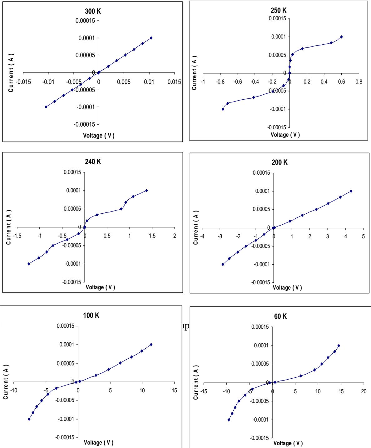
**Figure 6.2.1** IV characteristics at different temperatures of FeSi film deposited with  $0.71 \text{ J/cm}^2$  laser fluence
