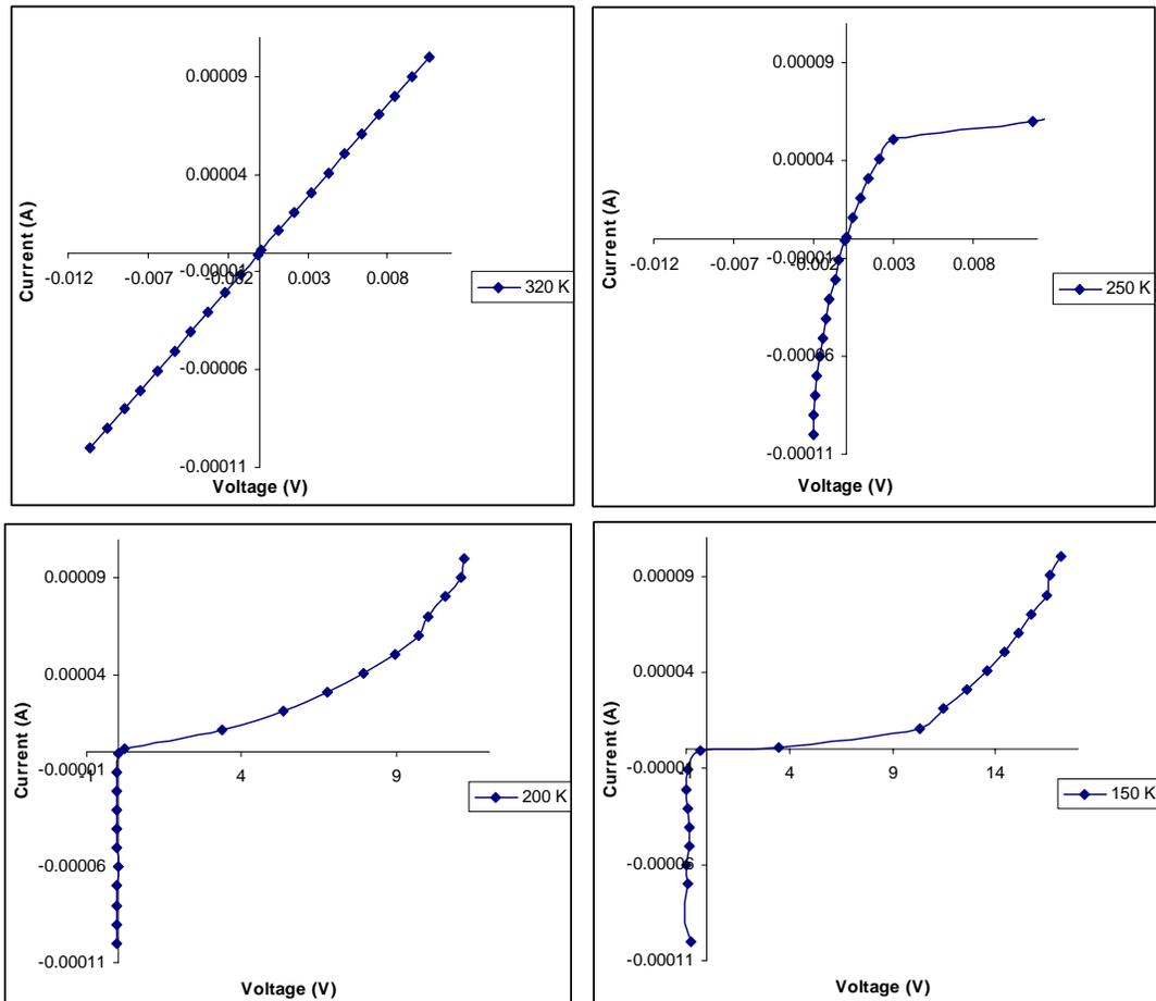
**Figure 5.2.1** IV curves of an isolated FeSi/SiO<sub>2</sub>/Si (*p*-type) system taken at different temperatures
