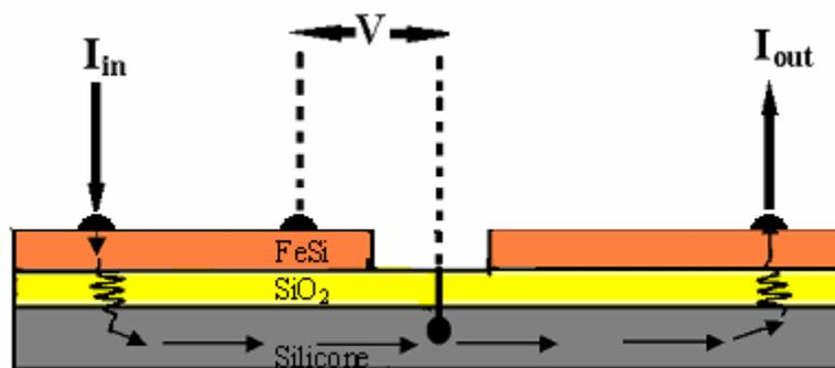
**Figure 5.1.7** Schematic diagram of the voltage probe placement for isolated FeSi/Si interface.
