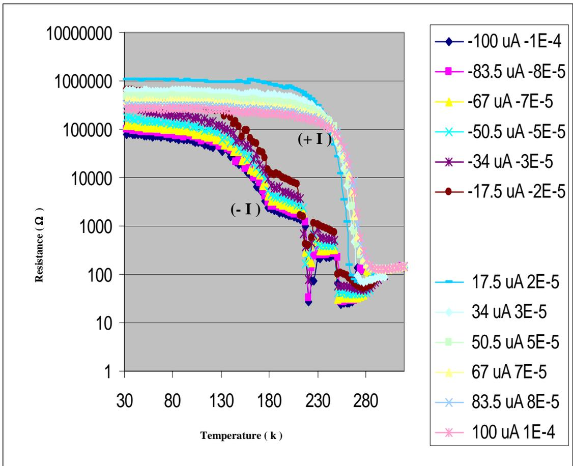
**Figure 5.1.8** Temperature dependence of the resistance for an isolated FeSi/Si interface of a FeSi deposited film on *p*-type substrate.
