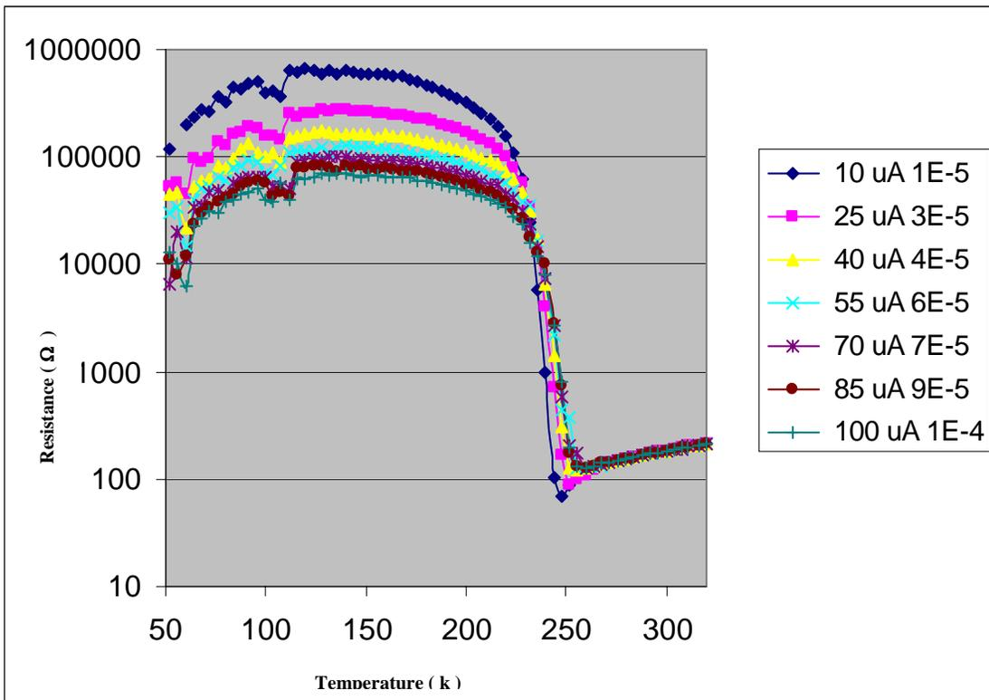
**Figure 5.1.1** The resistance of FeSi films deposited on *p*-type Si depending on temperature for different applied current values.
