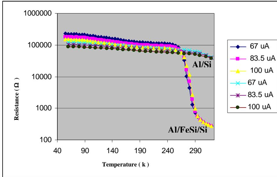
**Figure 5.4.4** The temperature dependence of resistance of discontinuous Aluminum coated and Aluminum coated FeSi deposited films on silicon substrates.
