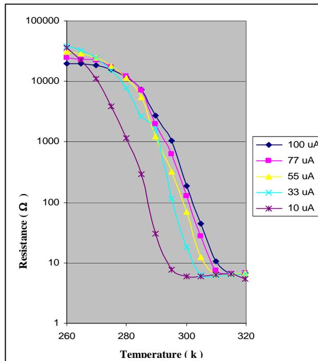
**Figure 5.1.4** Current dependence of the resistance change for a film on a *n*-type substrate near the transition
