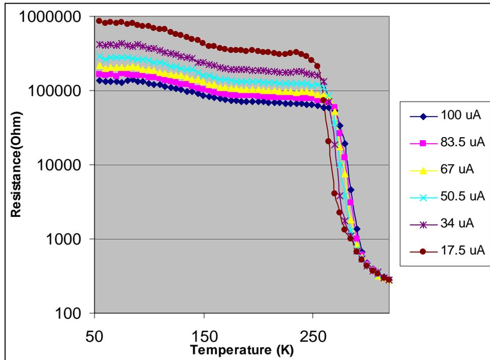
**Figure 5.1.6** Temperature dependence of the resistance for discontinuous FeSi deposited film on *p*-type substrate
