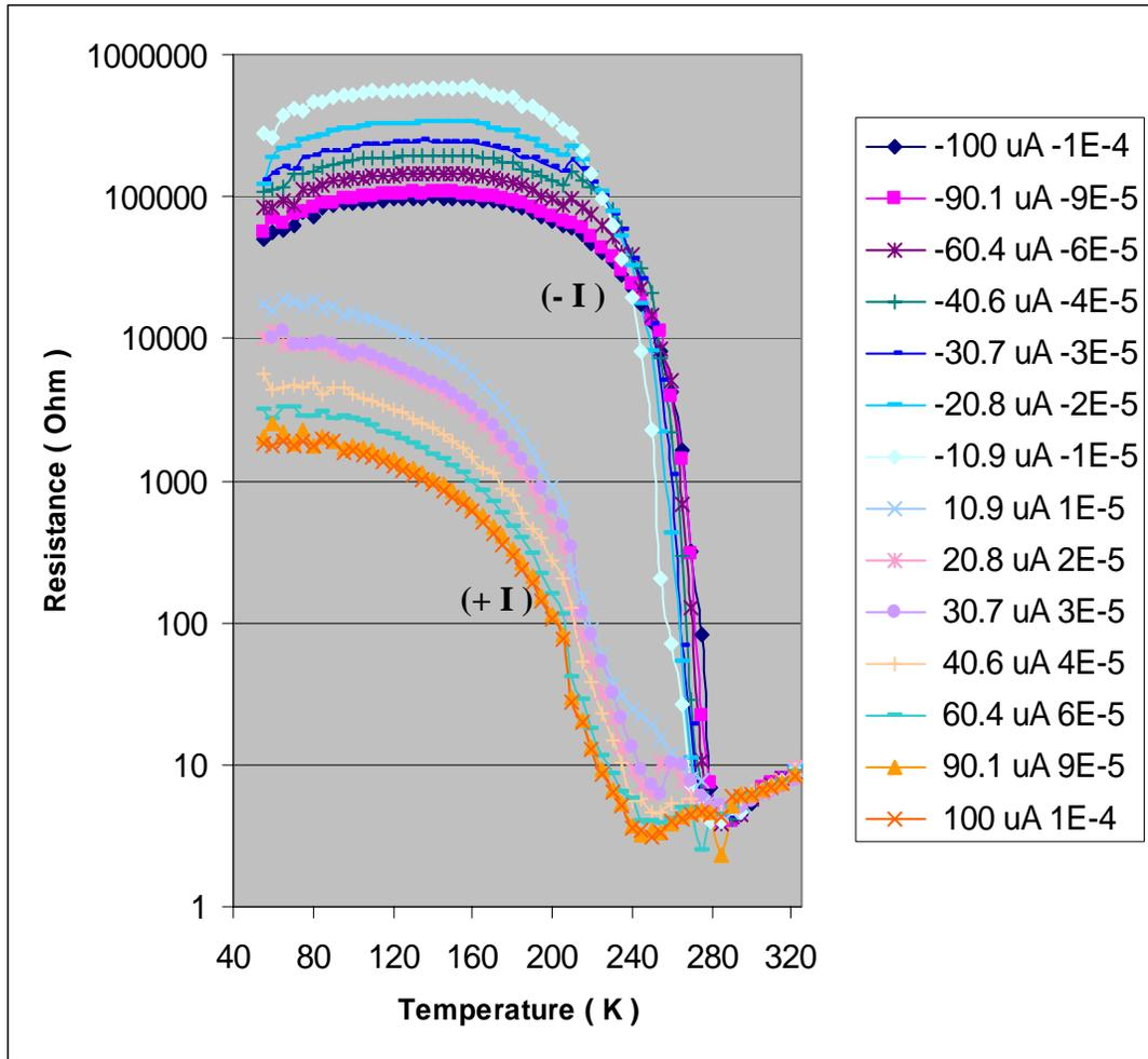
**Figure 5.1.9** Temperature dependence of the resistance for an isolated FeSi/Si interface of a FeSi deposited film on *n*-type substrate.
