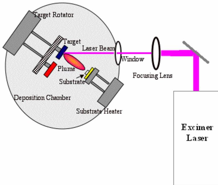
**Figure 3.1.1** The PLD system used to deposit the Iron Silicide films.
