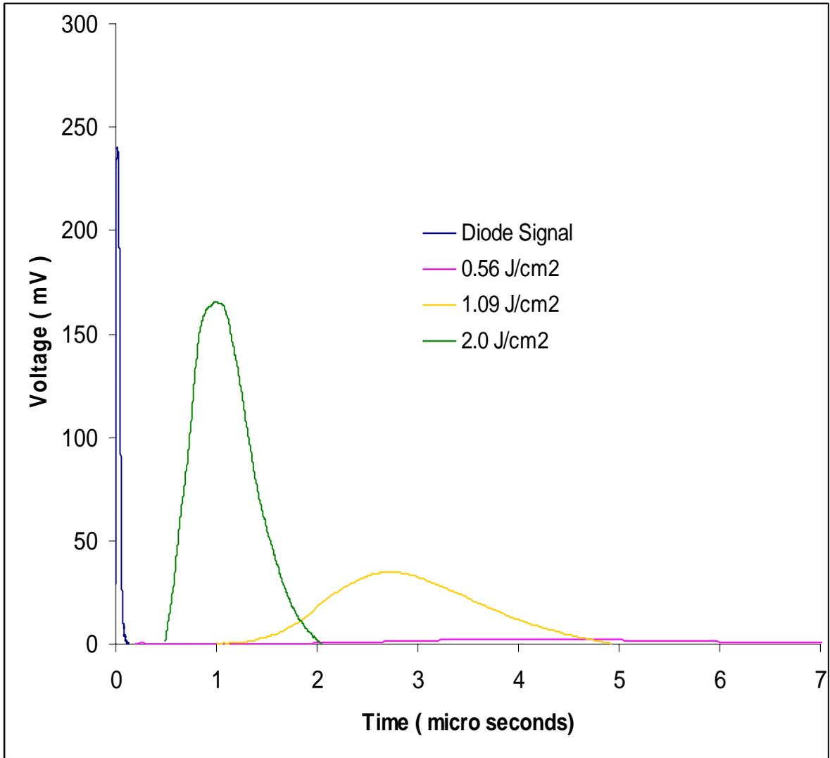
**Figure 6.3.3** The diode signal and the time-of-flight ion profiles obtained at different laser fluences.
