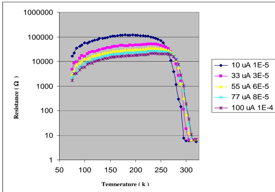
**Figure 5.1.2** The temperature dependence of resistance of PLD-deposited FeSi films on n-type Si, for applied different current values
