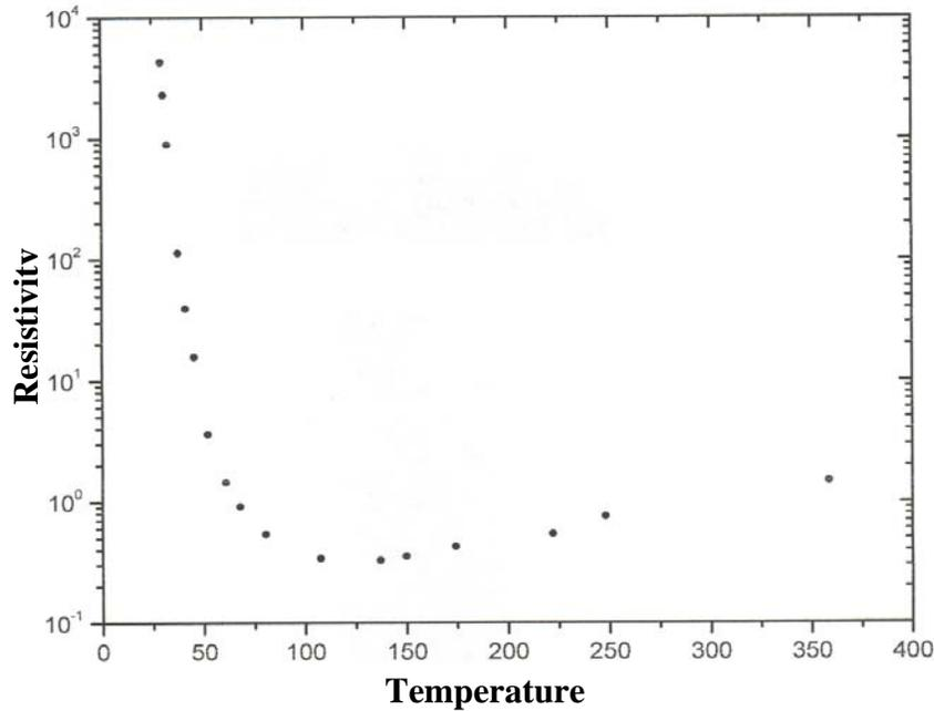
**Figure 3.2.2:** Resistivity depending on temperature for the Boron-doped p-type Si (Boron concentration in the sample is  $\sim 10^{15}$  atoms/cm<sup>3</sup>).
