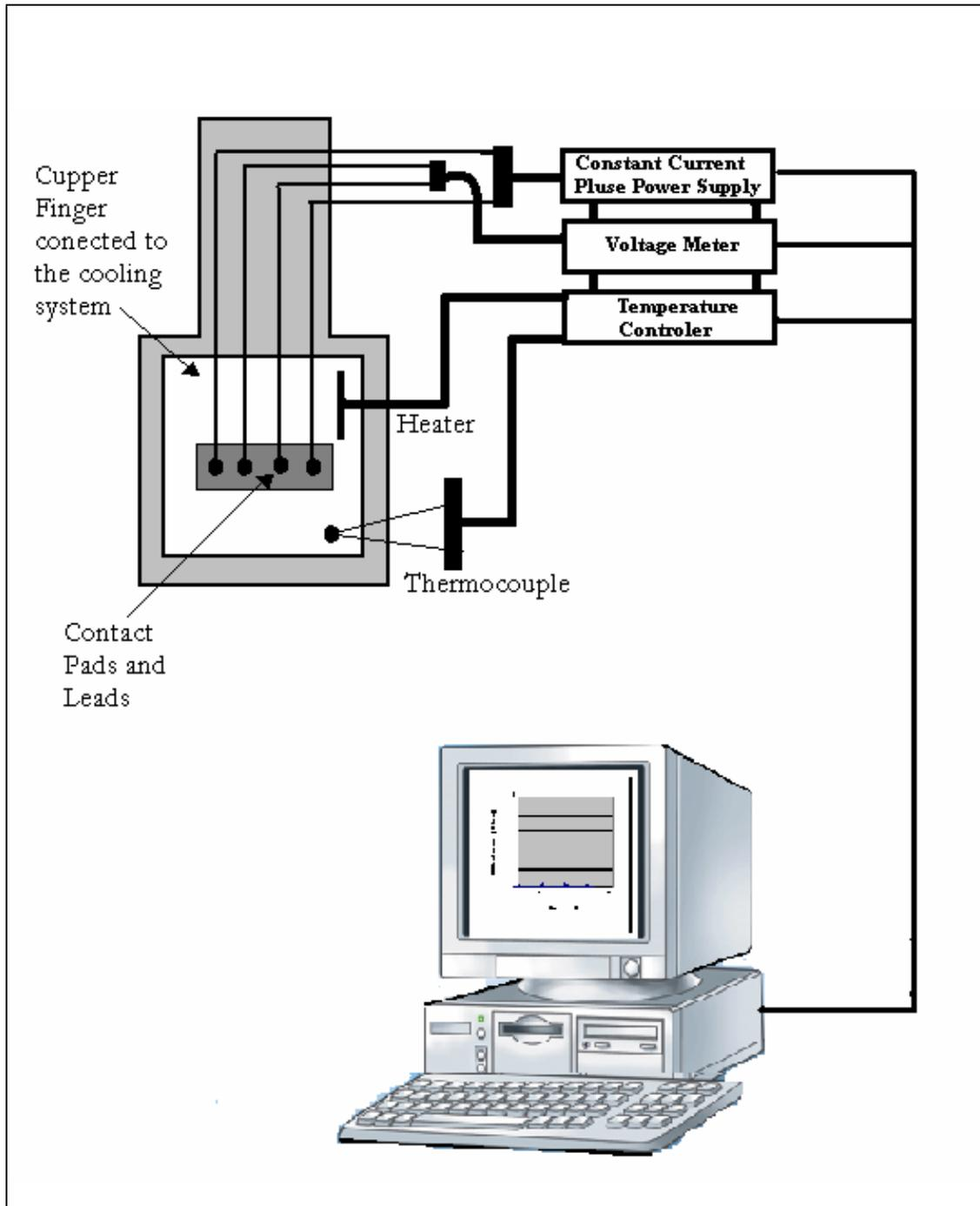
**Figure 4.1.3** Schematic diagram of the temperature dependant resistance measurement system. A PC through a GPIB connection to the different devices controlled the measurement process, from applying the current pulse to measuring the voltage during the given temperature range.
