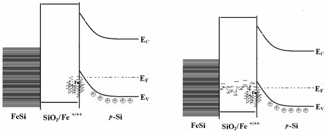
**Figure 7.1.2** Accumulation and carrier hopping through the  $\text{SiO}_2$  layer
