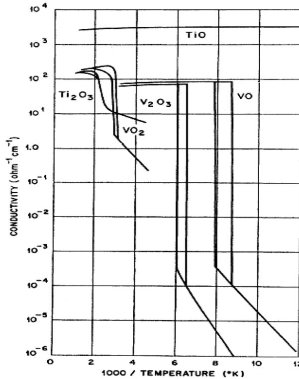
**Figure 1.1.1** Metal-to-insulator transition observed in different metal oxide systems. [N. F. MOTT (1968)]
