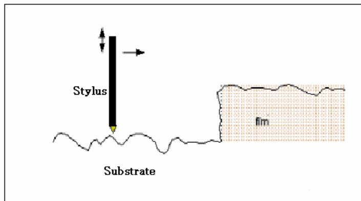
**Figure 4.1.1:** Principle of the Profilometer
