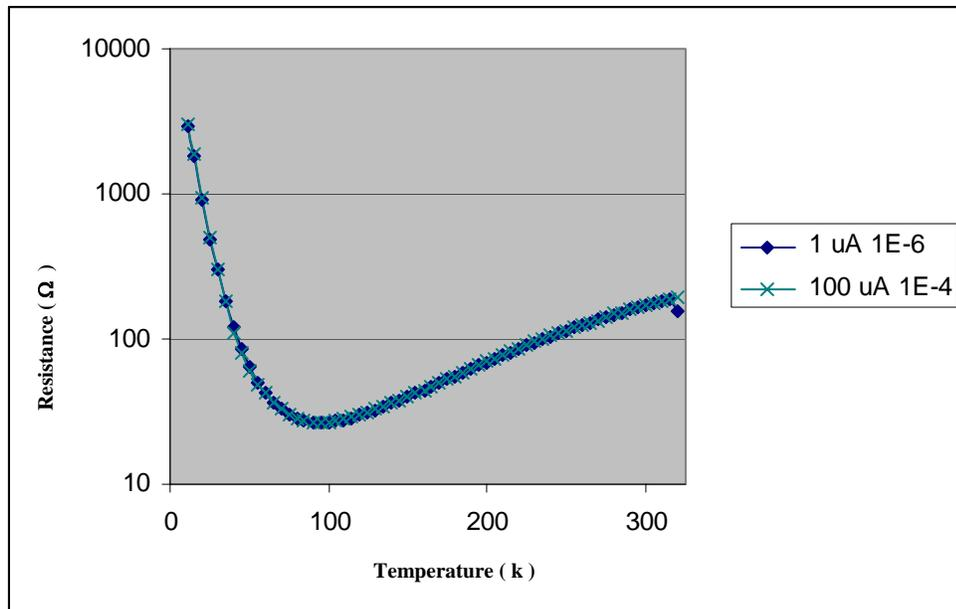
**Figure 5.4.5** The temperature dependence of resistance of discontinuous Aluminum coated after annealing at 450 °C for 30 minutes.
