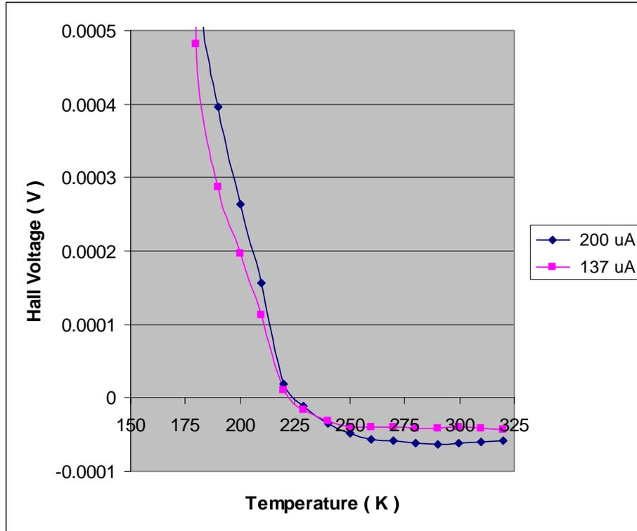
**Figure 5.3.3** Hall voltage dependence on temperature for FeSi deposited on *n*-type silicon substrate measured for two different current values.
