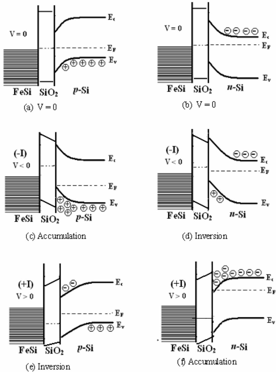
**Figure 7.1.3** Energy band bending for various applied potentials for FeSi/SiO<sub>2</sub>/Si systems.
