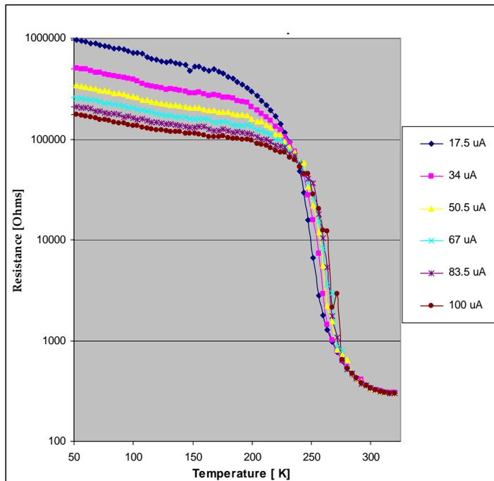
**Figure 5.4.3** The resistance dependence on temperature of and Pt/FeSi/SiO<sub>2</sub>/Si-*p* structure
