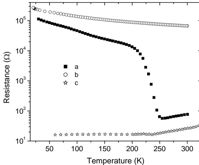
**Figure 1.1.1** Temperature dependence of the resistance of FeSi films deposited at 400°C on (a) p-type silicon substrate of resistivity 1- 10 Ω-cm, (b) sapphire substrate. Curve (c) shows the temperature dependence of resistance for the etched silicon substrate. [S.Withnachchi. et all (2006)]
