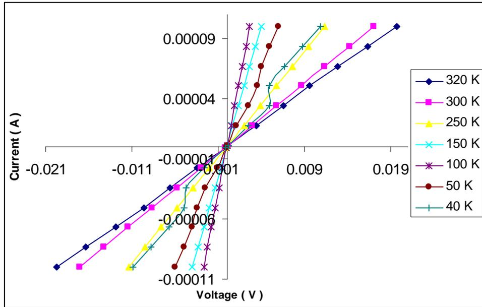
**Figure 5.4.6** IV curves of annealed discontinuous Al/Si system taken at different temperatures
