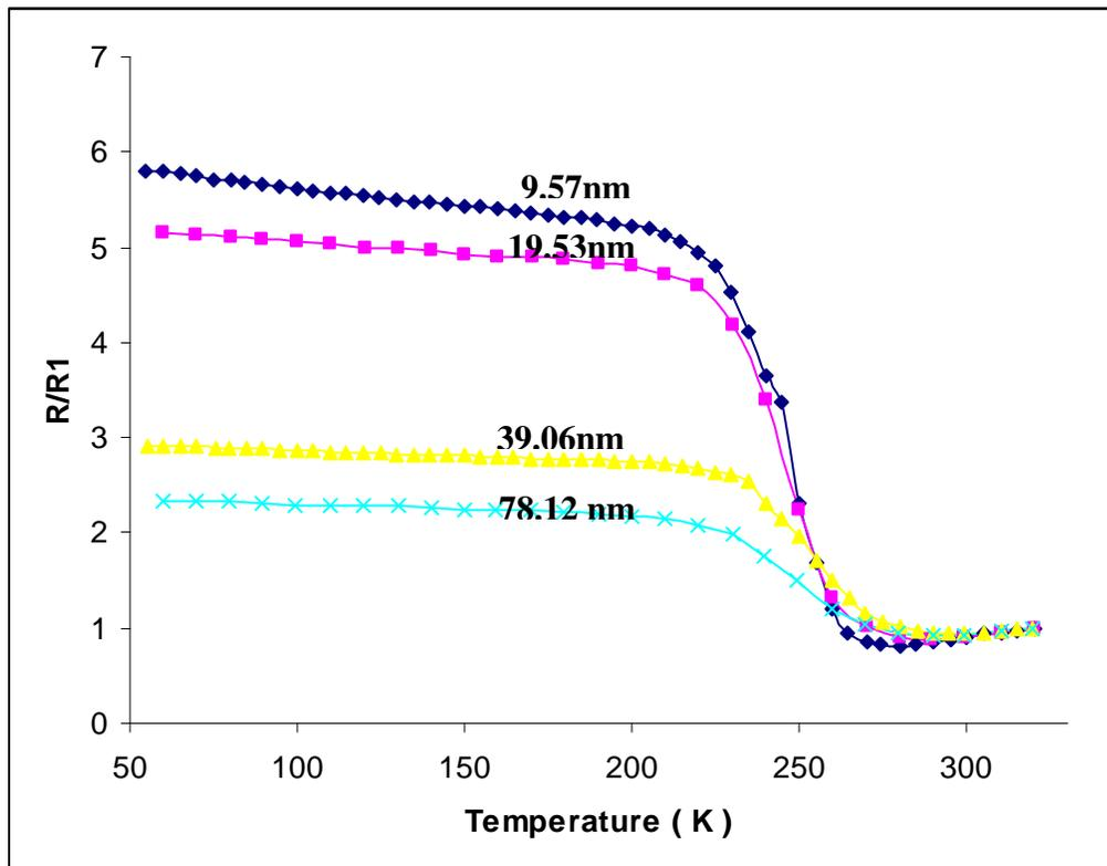
**Figure 6.4.1** Thickness dependence on the transition FeSi films deposited at high fluence ( $3.5 \text{ J/cm}^2$ ).
