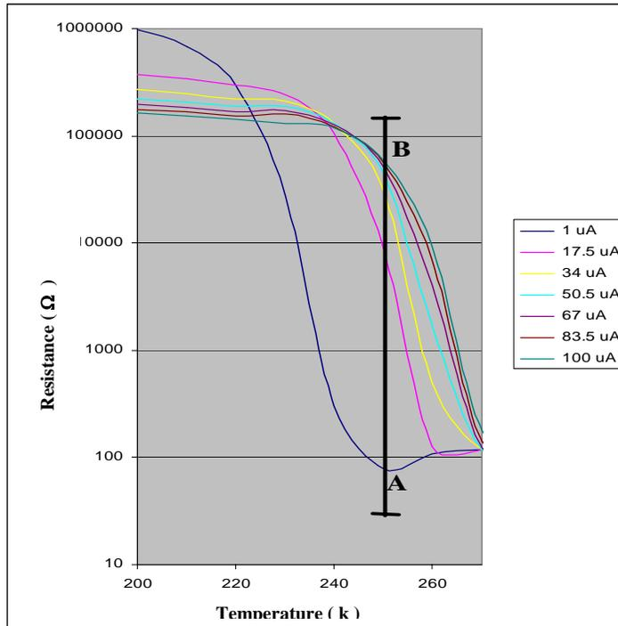
**Figure 5.1.3** Current dependence of the resistance change for a film on a *p*-type substrate near the transition
