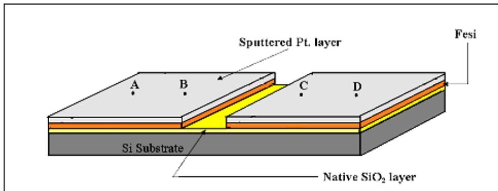
**Figure 5.4.1** Schematic diagram of the fabrication procedure of FeSi films with sputtered platinum layer.
