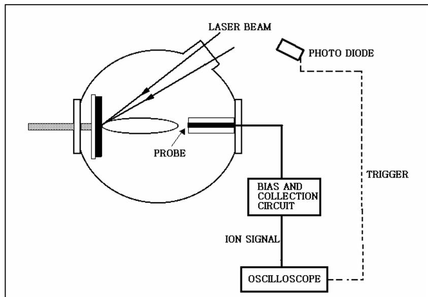
**Figure 6.3.1** schematic diagram of the ion probe set up.
