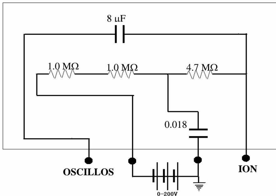
**Figure 6.3.2** Bias and collecting circuit used
