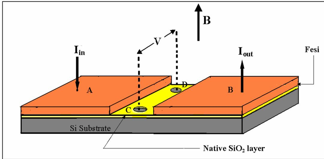
**Figure 5.3.1** Schematic diagram of the current and voltage probe placement for Hall voltage measurements.
