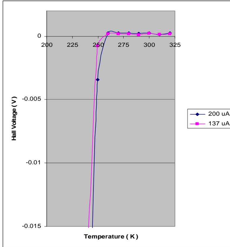
**Figure 5.3.2** Hall voltage dependence on temperature for FeSi deposited on p-type silicon substrate measured for two different current values.
