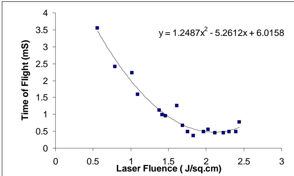
**Figure 6.3.5** Fluence dependence of time-of-flight
