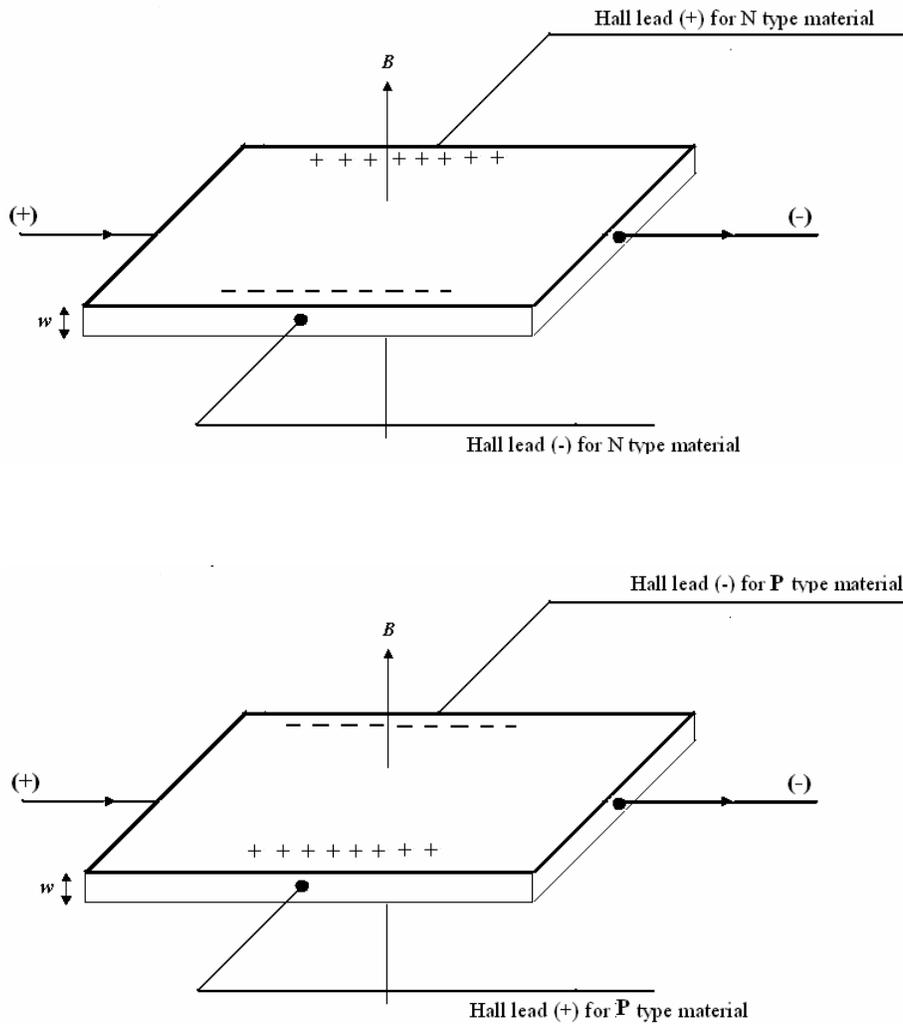
**Figure 4.2.1** Basic principle used to identify the carrier type (sign convention)
