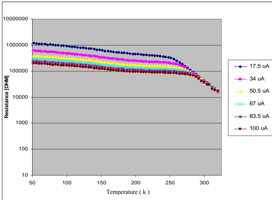
**Figure 5.4.2** The resistance dependence on temperature of and Pt/SiO<sub>2</sub>/Si-*p* structure
