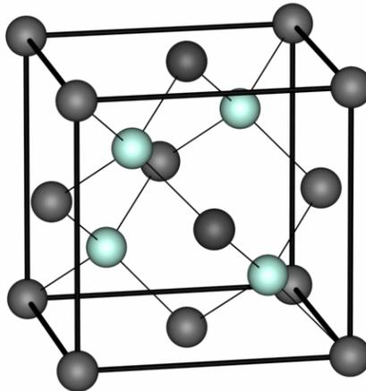
**Figure 3.2.1** Silicon crystallographic structure. It has the diamond structure, which is two fcc structures shifted along the diagonal with respect to each other
