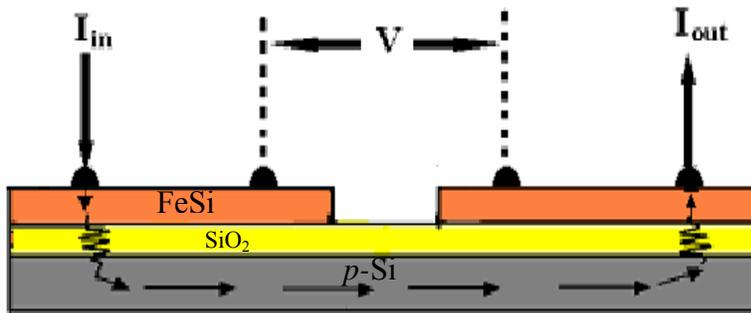
**Figure 5.1.5** Schematic diagram of the voltage probe placement for isolated FeSi/Si interface
