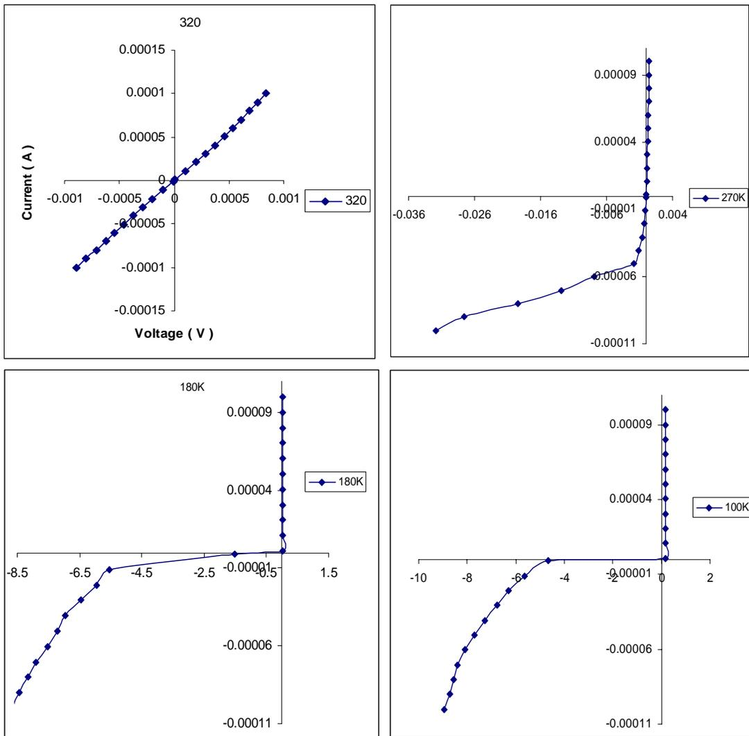
**Figure 5.2.2** IV curves of an isolated FeSi/SiO<sub>2</sub>/Si (*n*-type) system taken at different temperatures
