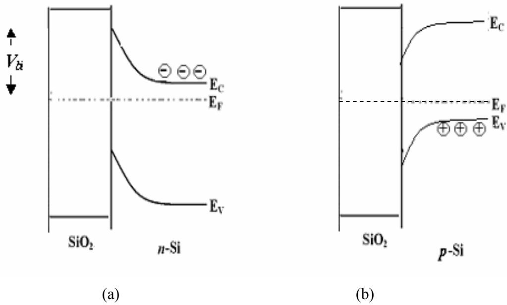
**Figure 7.1.1** Band bending  $\text{SiO}_2/\text{Si}$  interface for a)  $n$ - and b)  $p$ -type substrates.
