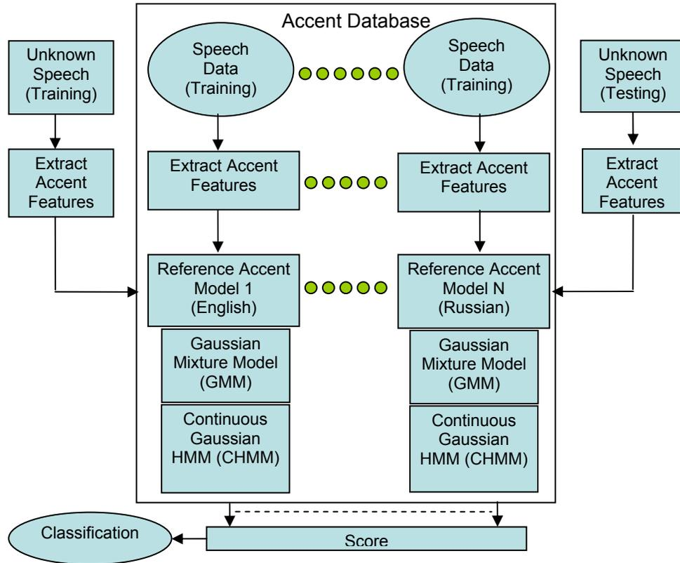
Figure 17. Block Diagram of Accent Classification (AC) System
