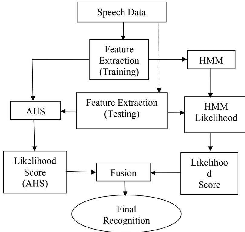
Figure 6. Flow Chart for Hybrid Fusion (HF) System
