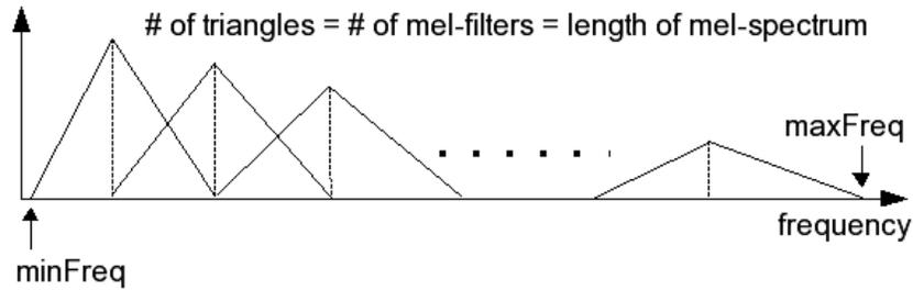
Figure 14. Mel-Spaced Filters
