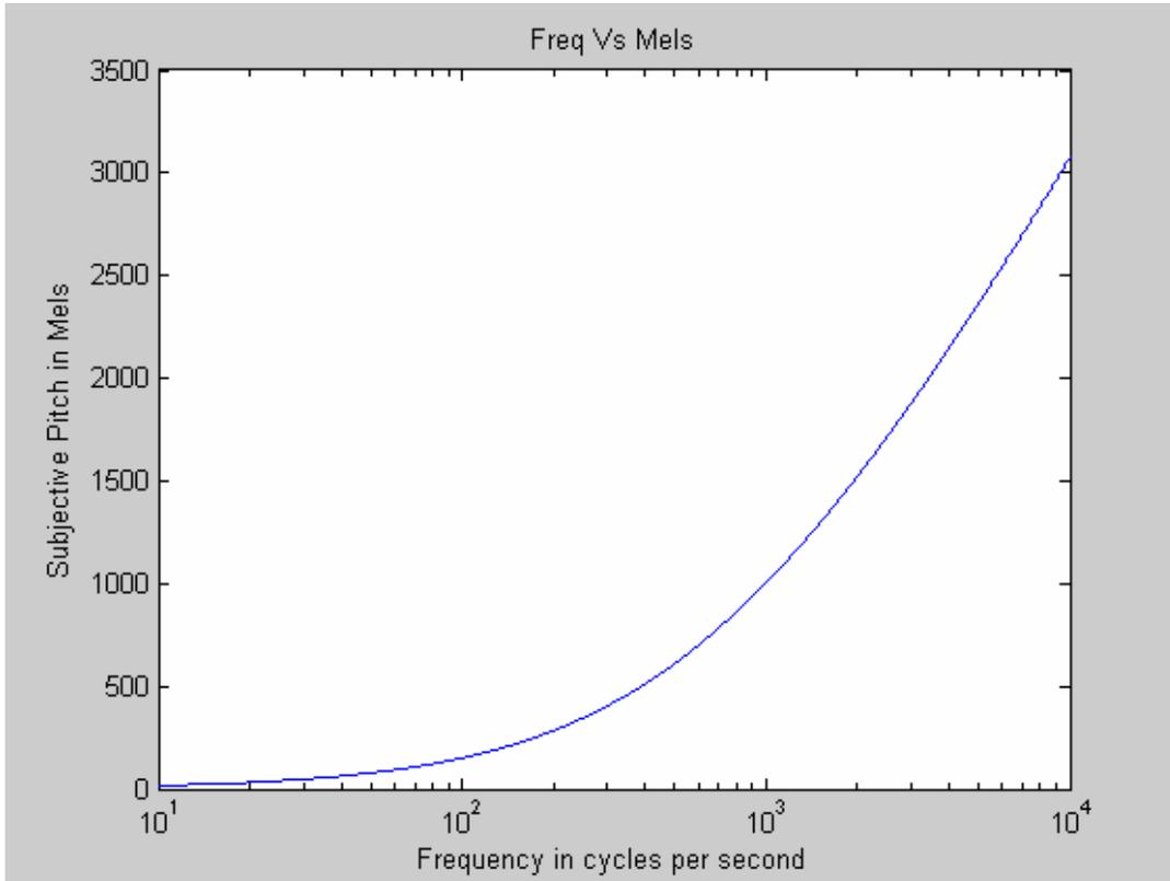
Figure 13. Frequency Mapping Between Hertz and Mels
