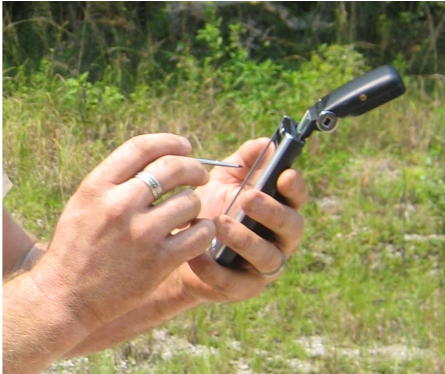
Figure 16. Mobile GPS unit linked with PDA device for acquisition of cave locations (photo by Jason Polk).
