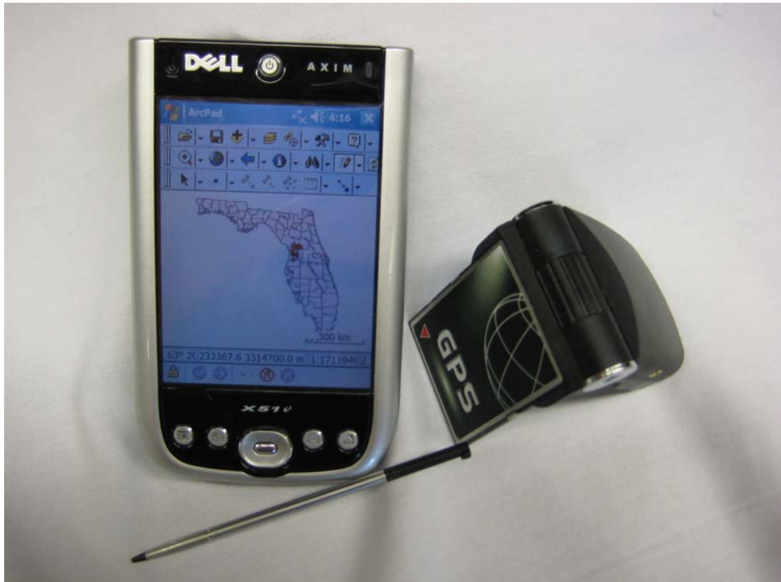
Figure 14. The tools used for inventory data collection in the field included ArcPad 7.1 GIS software, Dell Axim PDA, and a mobile GPS device. ArcPad 7.1 was loaded onto a Dell Axim PDA. A PDA and a mobile Global Positioning System (GPS) unit, which plugged directly into the PDA, were used for inventory data collection in the field.
