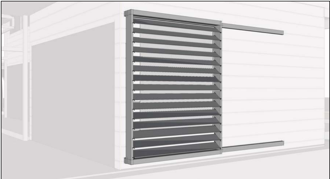
Fig.14 Solar adjustable louver system, it can also be moved to the side of the window opening if sun light is desired inside the building.
