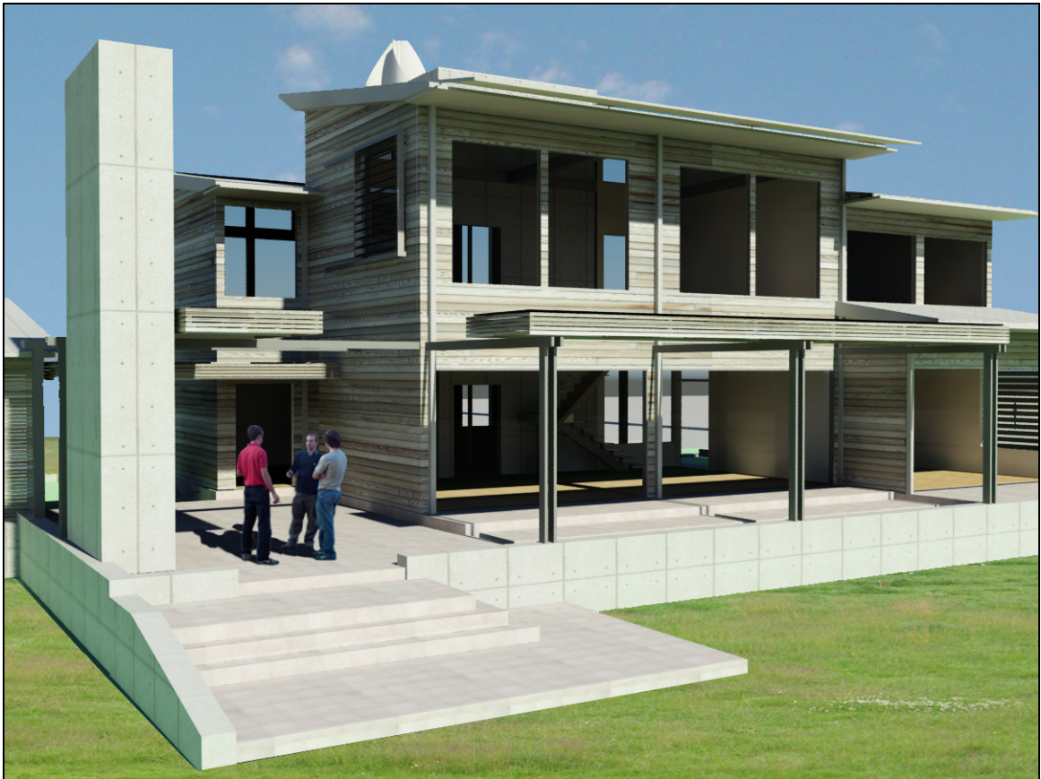
Fig.76 South west perspective. Adjustable arrays set for winter allowing heat gain to interior.
