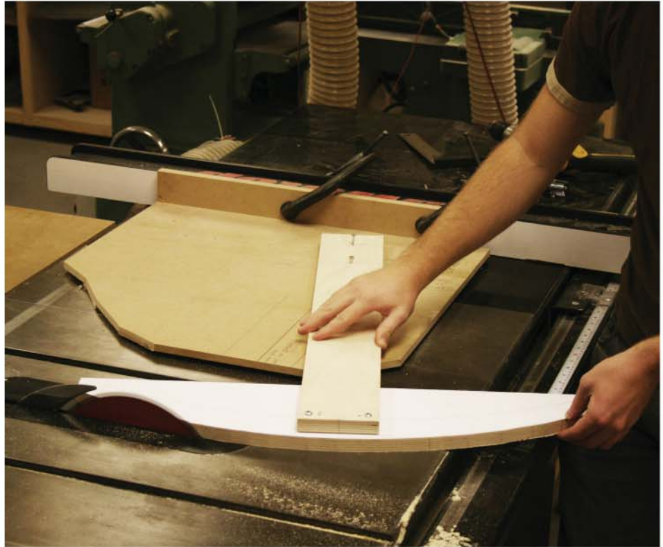
Fig. 59. Cutting compound curve with jig
