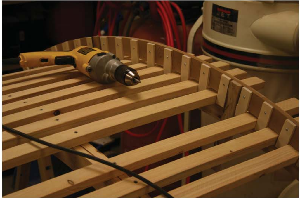
Fig.80. Wall Section Model with assembly jig attached
