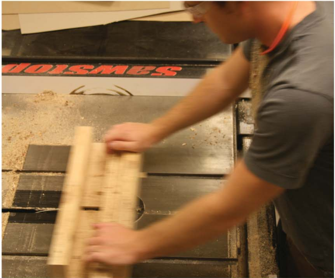
Fig. 25. Cutting With Dado
