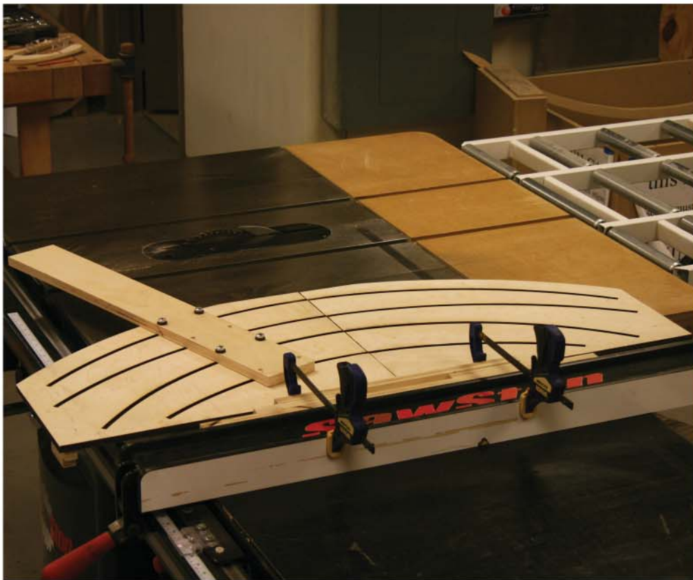
Fig. 110. Jig clamped to table saw
