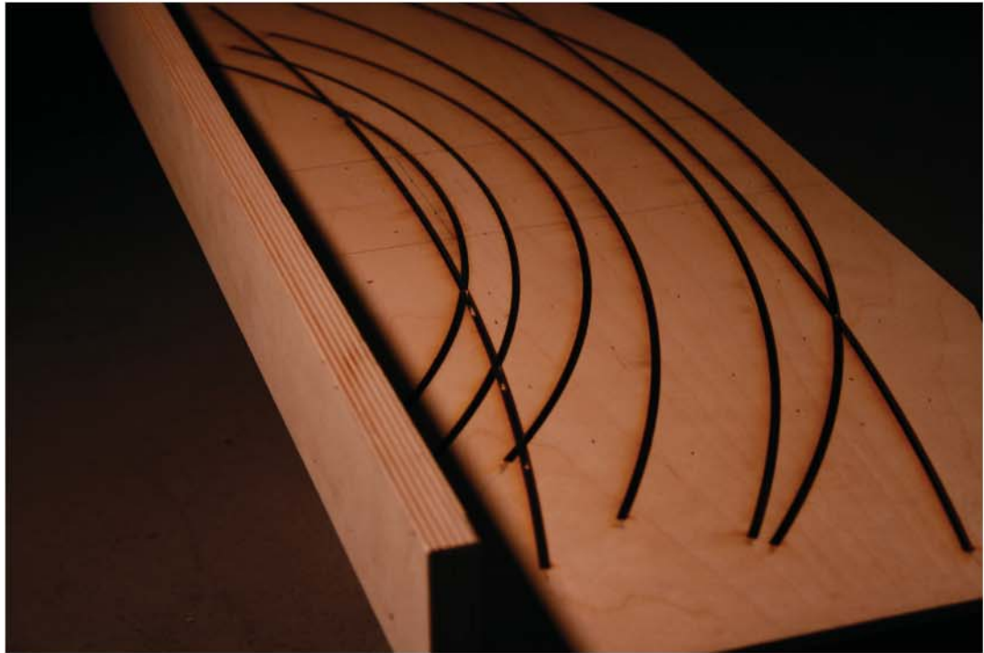
Fig. 51. Jig designed to cut multiple radius curves
