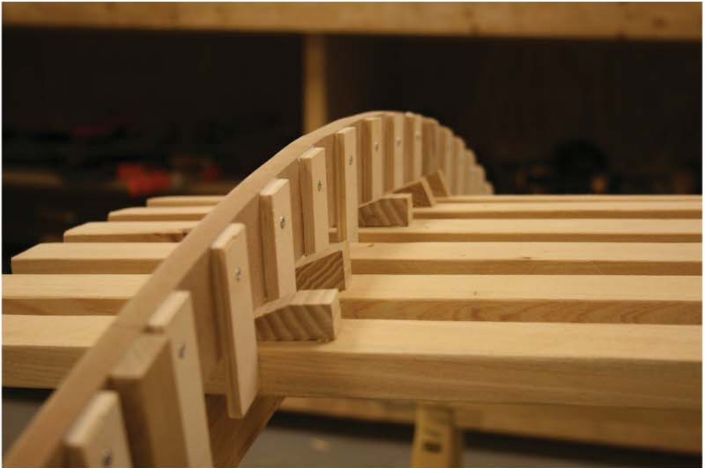
Fig. 81. Wall Section Model with assembly jig attached
