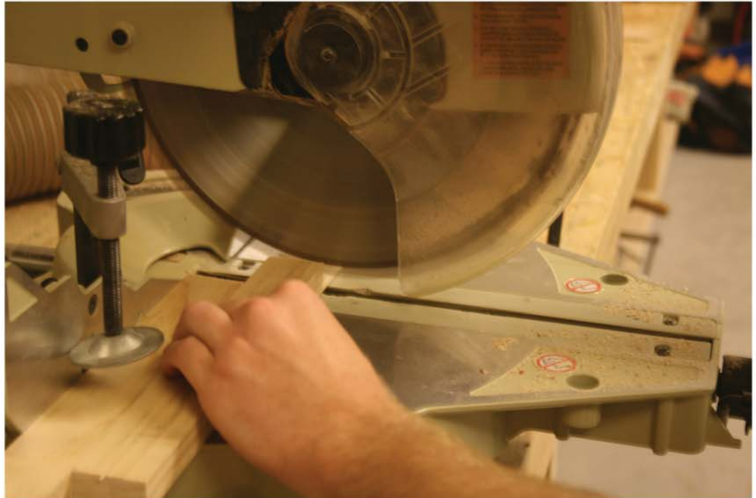
Fig. 17. Cutting Half Lap
