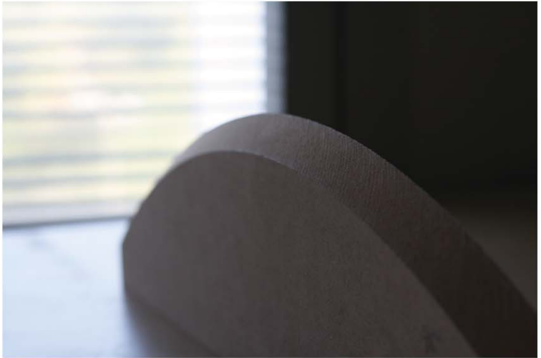
Fig. 50. Texture left from blade
