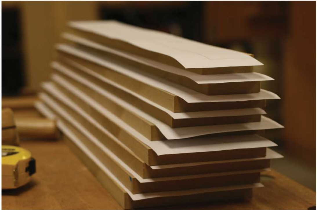
Fig.47. MDF strips with mounted autocad prints
