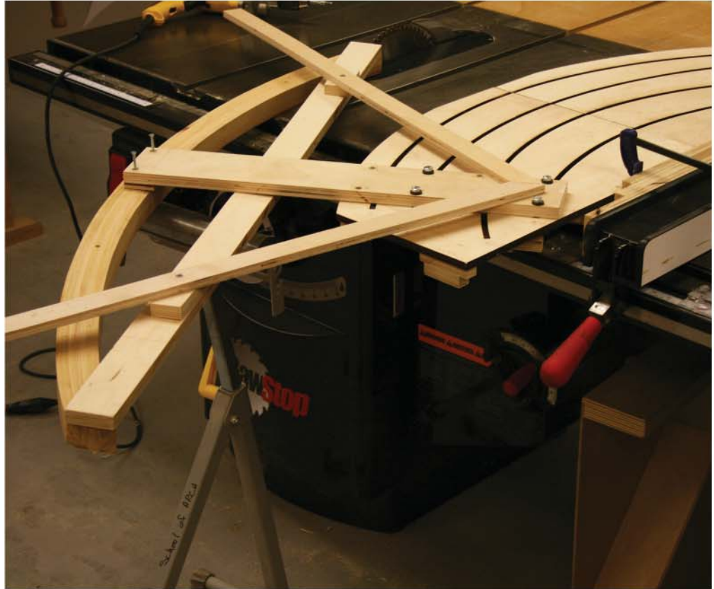
Fig. 112. Glu Lam ready to be cut
