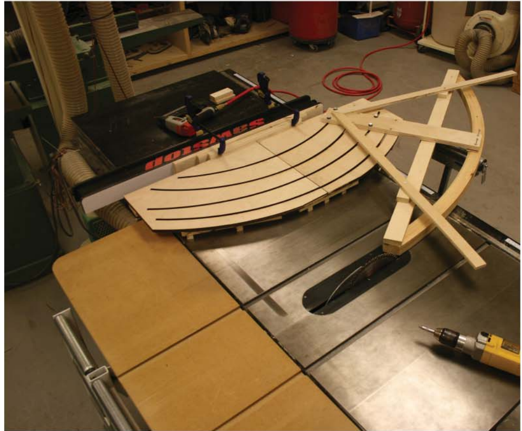
Fig. 111. Trammel arm sliding on jig
