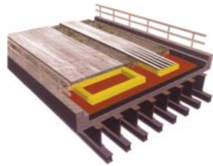
Figure 2.14 - Modular planking and planting system adds a rich variety to the horizontal plane of the park. (Source: Online)
