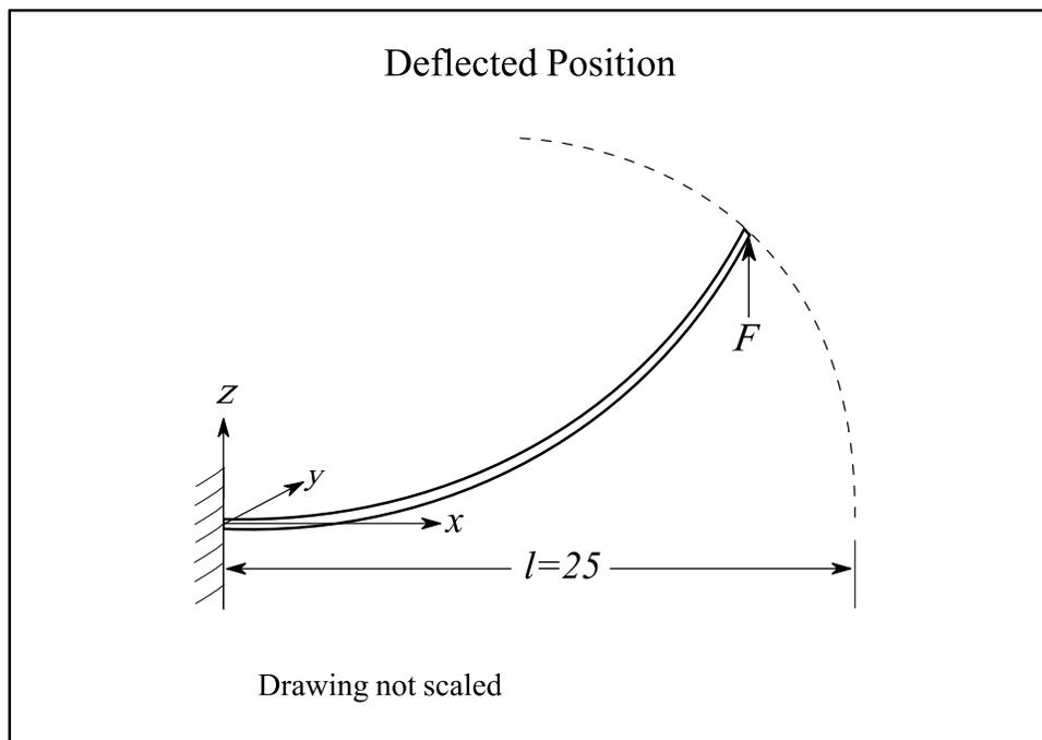
Figure 3.2. Shows the deflected position of beam Case 1.
