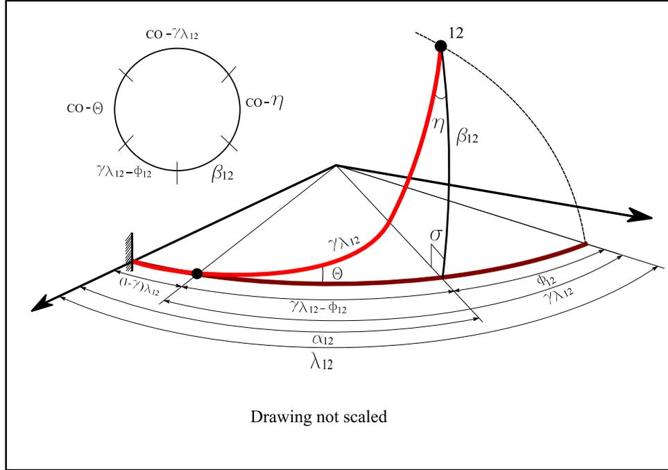
Figure 3.19. The spherical right triangle formed by a curved beam.
