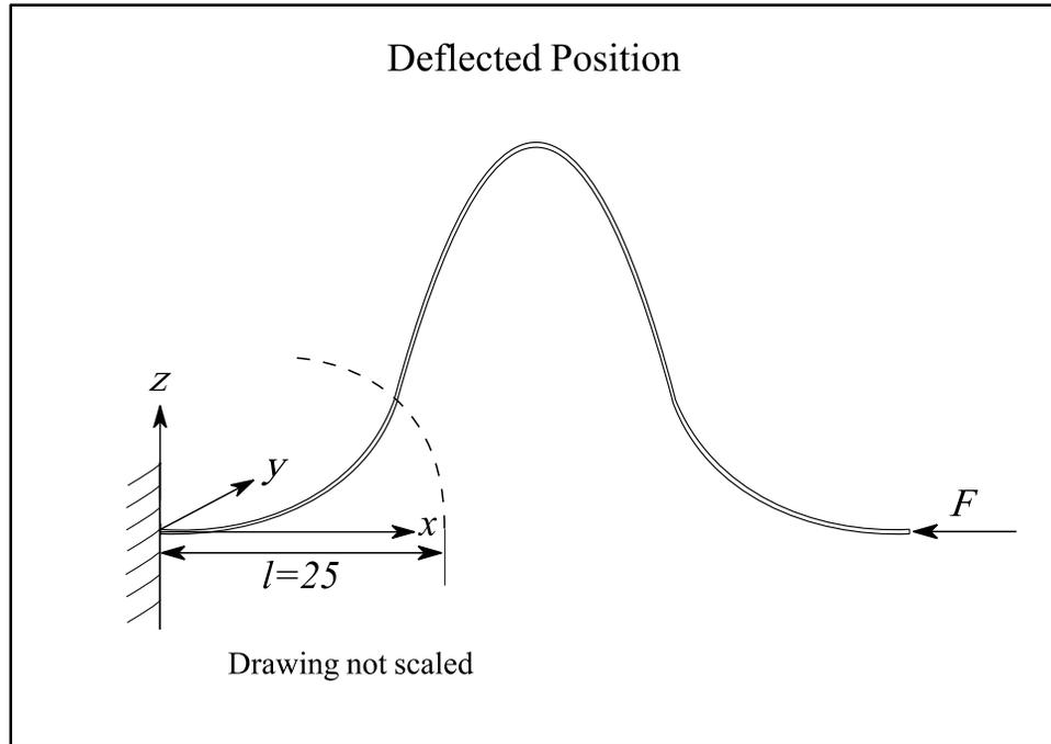
Figure 3.4. Shows the deflected position of beam Case 2.
