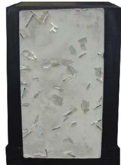
Figure 55. Model of transparent concrete (the interior view)
