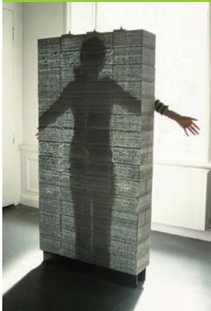
Figure 47. Transparent concrete
