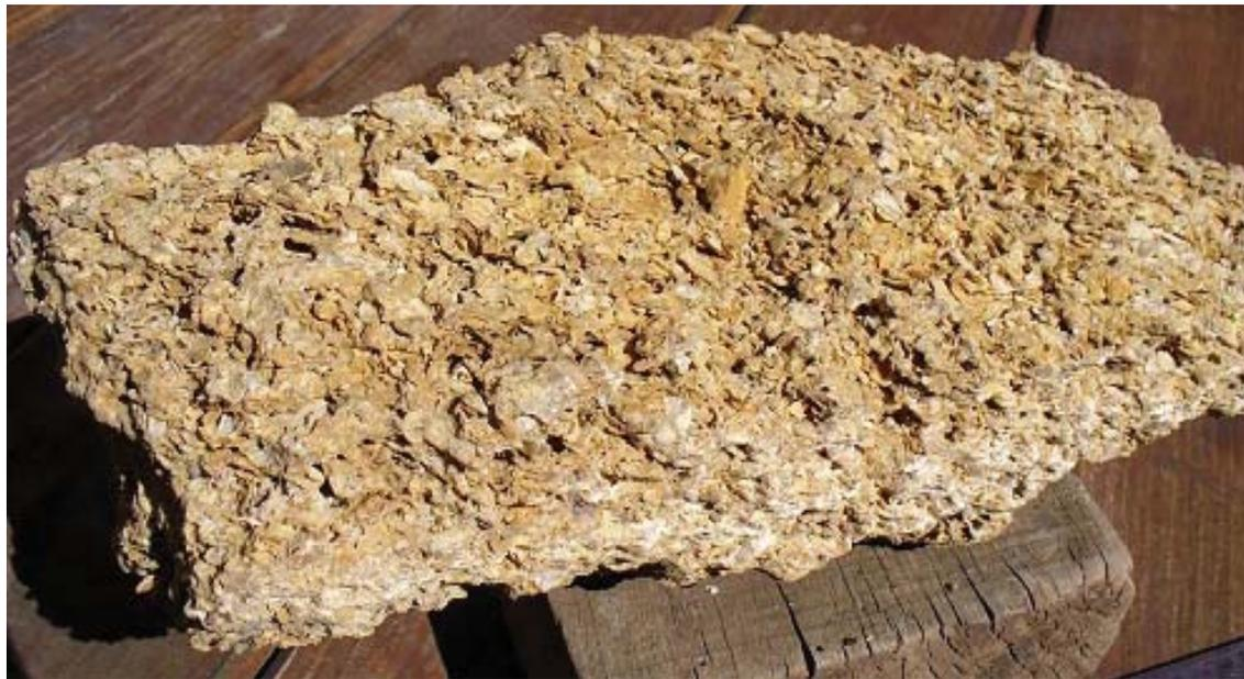
Figure 27. Image of the material 'coquina'
