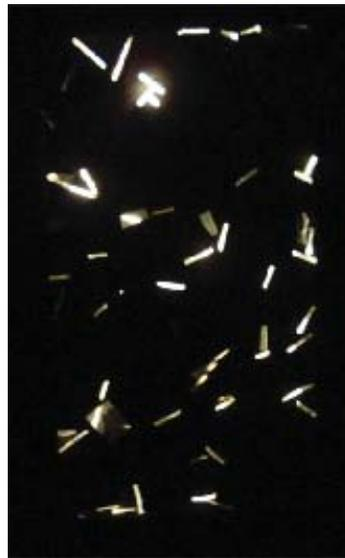
Figure 53. Model of transparent concrete with the lights off
