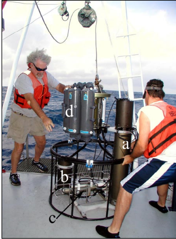
Figure 5. Deployment of the General Oceanic Rosette frame. On board were the following: a) UMS system b) batteries c) CTD d) Niskin water samplers.
