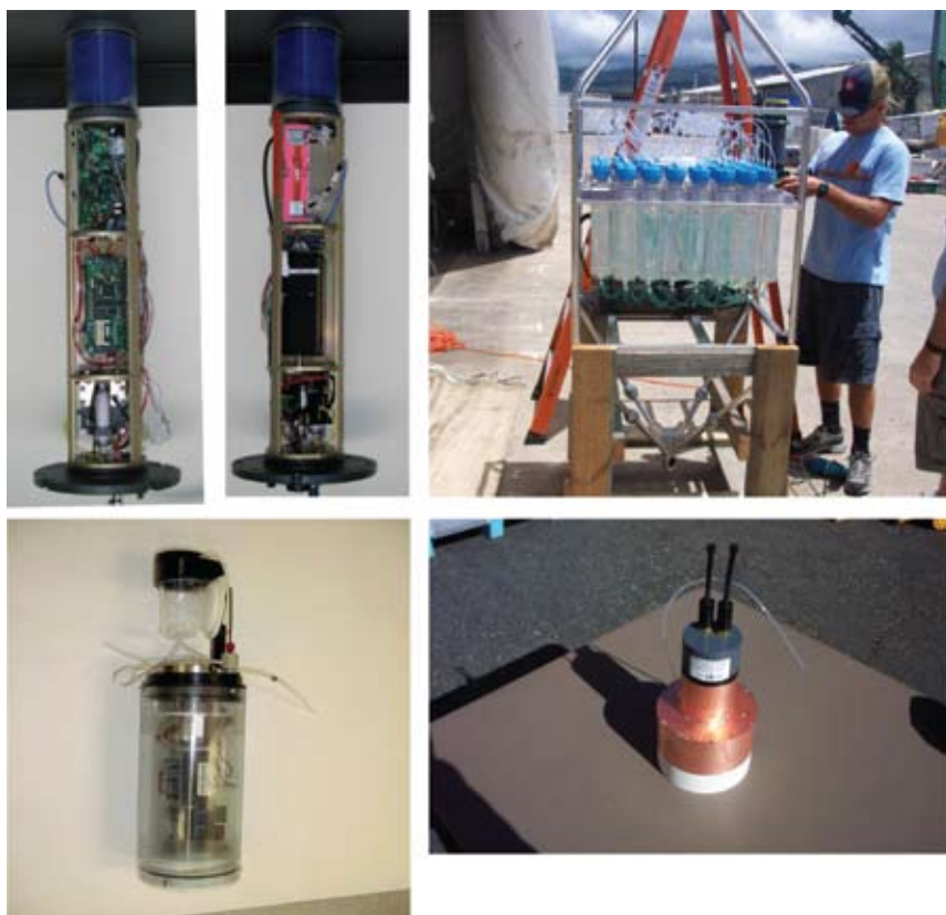
Figure 2. Chemical measurement systems used during the NOPP O-SCOPE and MOSEAN programs. (Upper left) Two views of the MAPCO 2 system that was deployed from the MOSEAN H-A buoy. (Upper right) The Remote Access Samplers (RAS) system deployed from the MOSEAN H-A buoy. (Lower left) The Spectrophotometric Elemental Analysis System (SEAS), which was deployed from the NOAA tsunami mooring. (Lower right) The SubChem phosphate analyzer deployed from the MOSEAN CHARM mooring.
