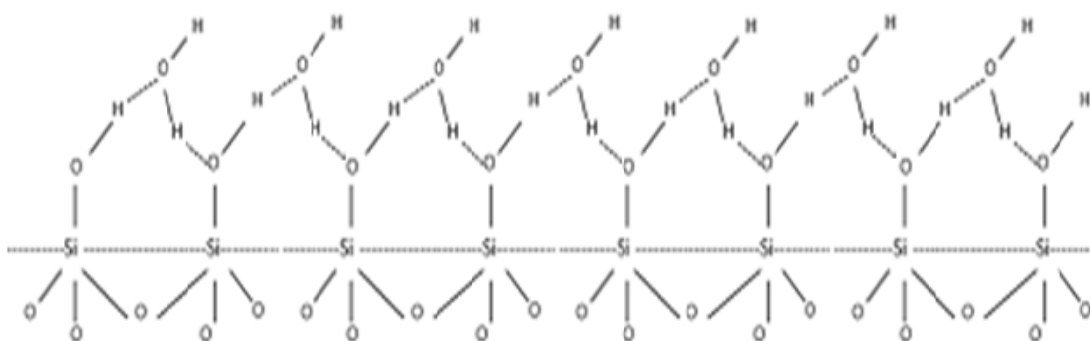
Figure 3. Silica surface surrounded by water molecule via multiple bonding
