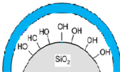
Figure 3. Silica surface surrounded by water molecule via multiple bonding
