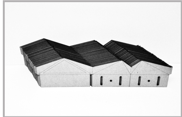
Fig.81. Lasercut chip board - the stacked cut out pieces of chip board prior to folding, stacked in a flat-pack manner
