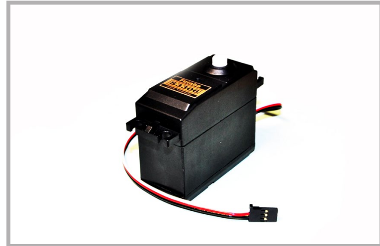
Fig.71. Individual servo motor - Futuba S3306 can provide 26Kg/ square inch of torque on 6v power
