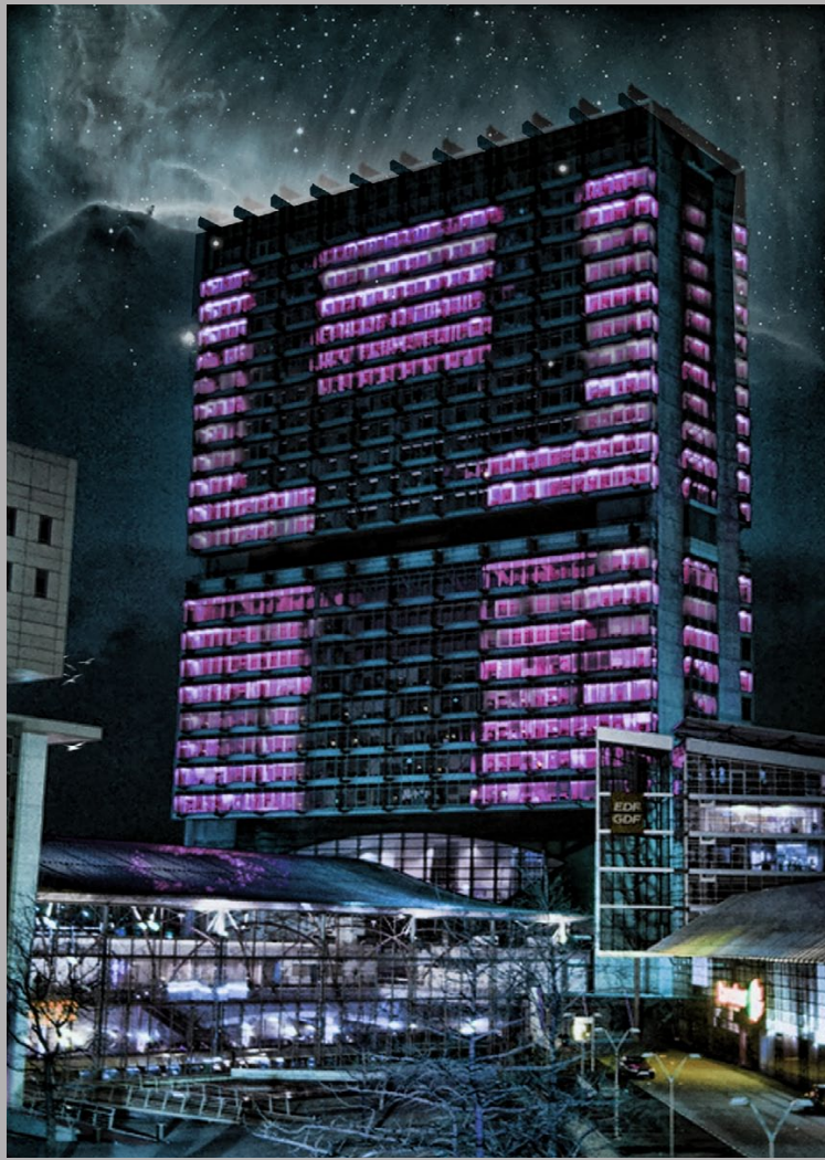
Fig.51. Conceptual rendering 3 - showing the time-based visual change that can be achieved with an individually controlled modular system
