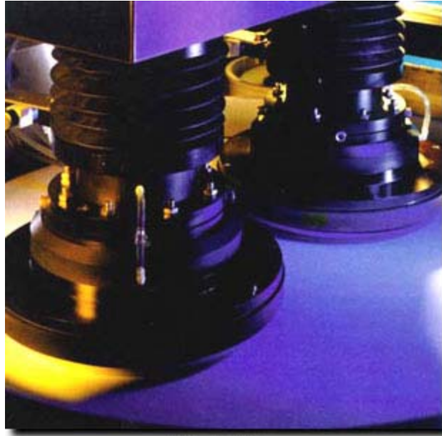
Figure 1.1: Integrated Circuit Wafer Polishing
