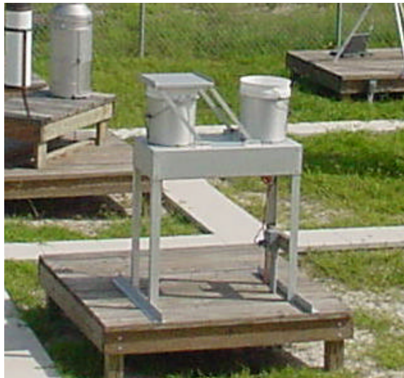
Figure 4. Photograph of Aerochem Metrics Model 301 wet/dry precipitation collector.
